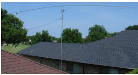
Photo E: Completed 17/12M trap dipole
