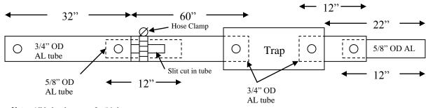
**Note:** All holes shown are for #6 sheet metal screws. Use 9/64"D clearance holes in fiberglass, 7/64"D clearance holes in AL tubing.
