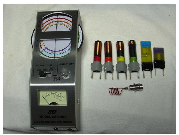
Photo D: The MFJ-201 Grid-Dip Oscillator
