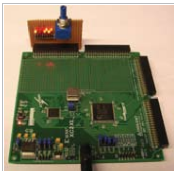
Figure 2 The application uses a Xilinx XC9500 XL CPLD.
