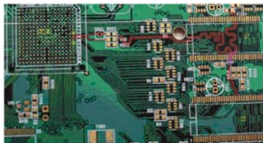
Figure 2 The bare PCB shows the differential-signal traces from the SOC to IC 1 and IC 2 .
