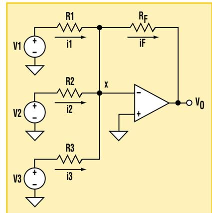
1. The traditional summing amplifier shown above has multiple inputs and one single-ended output.
