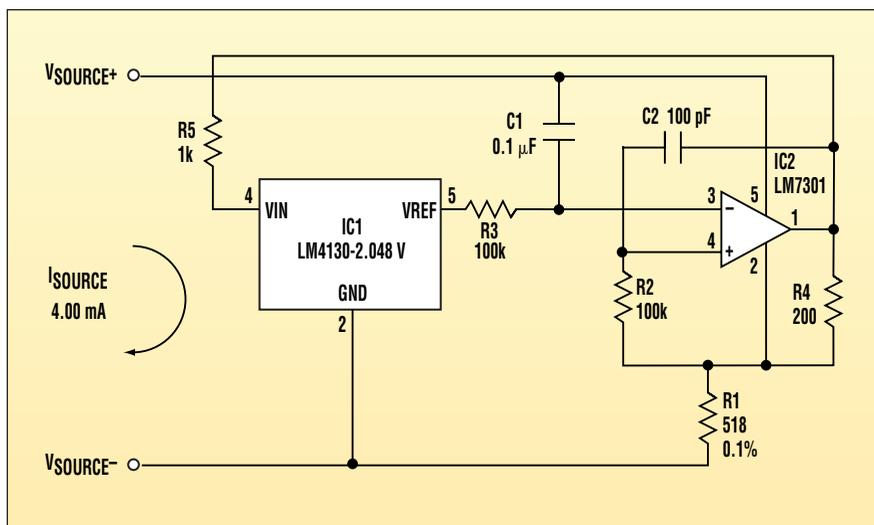
1. This composite CMOS voltage reference and op-amp integrator forms a general-purpose current source. The bootstrap configuration eliminates IC2's ground-current error.
