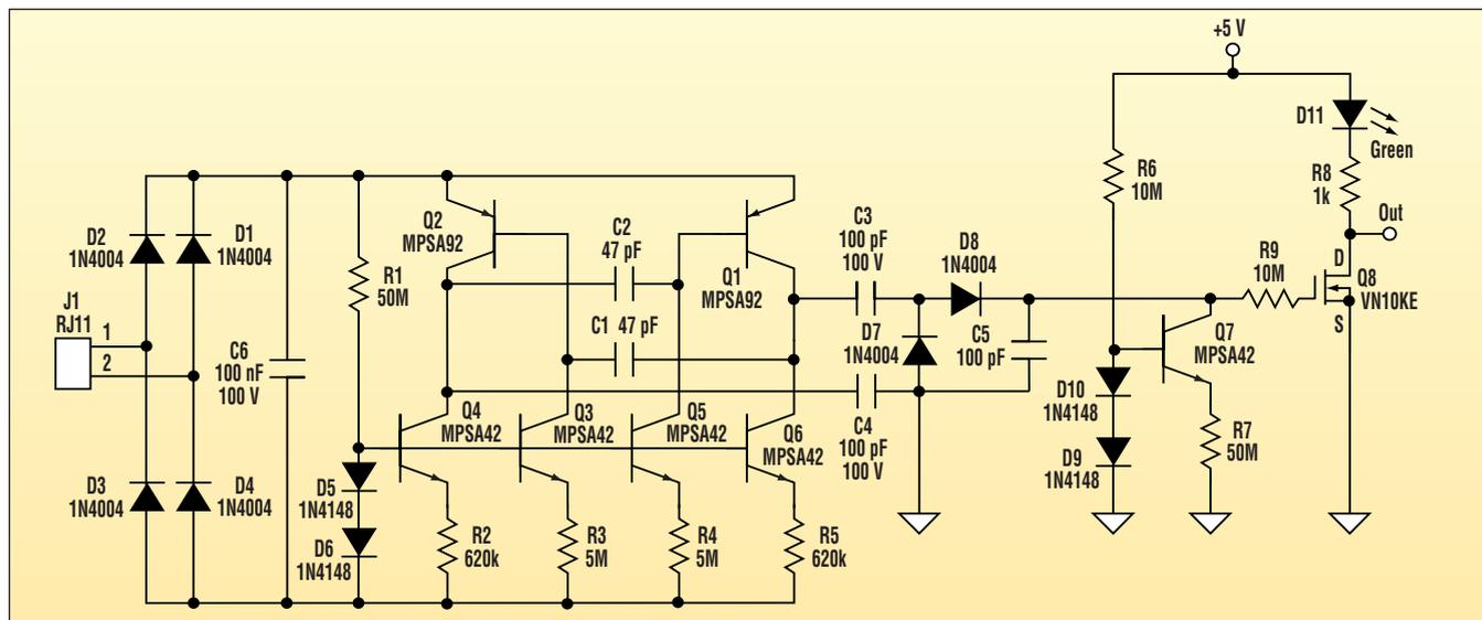
A micropower oscillator biased by the telephone line is coupled to an isolated detection circuit to detect possible breaks in the phone line.
