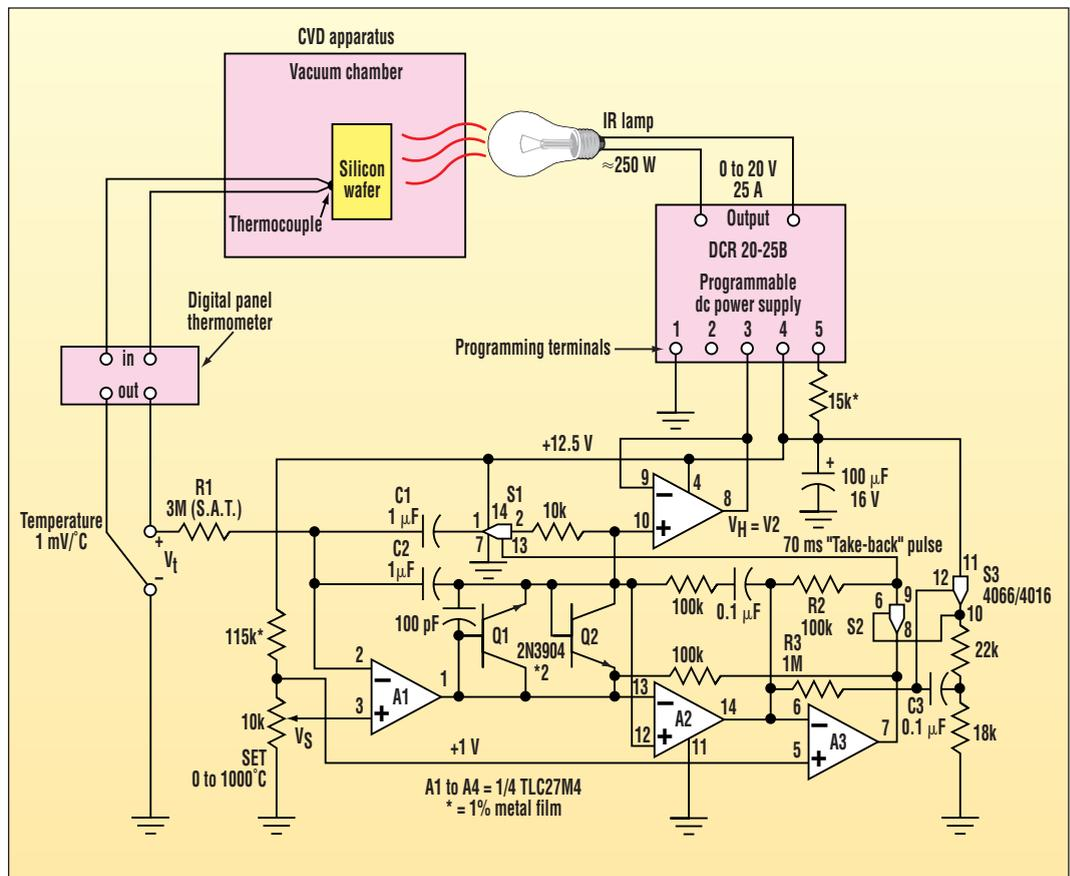
2. This circuit achieves accurate temperature control over a 100°C to 1000°C range by using a “Take-Back-Half” temperature-control algorithm, described in detail in an earlier Idea For Design.
