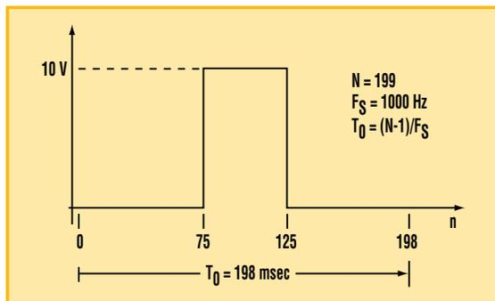
1. To demonstrate the program, an input 50-ms pulse was created and fed into the program.
