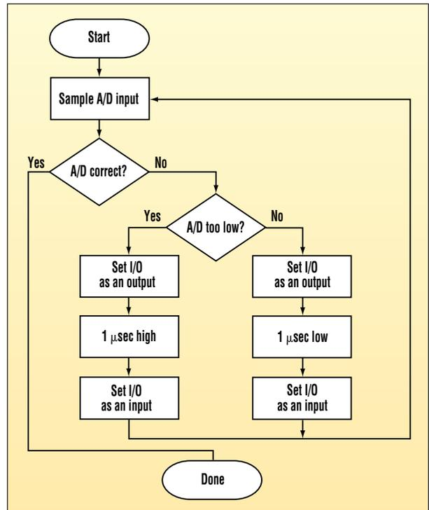
**2.** This simple algorithm can adjust the voltage across C1 at a rate of about 1 LSB per microsecond, allowing completion of a near-rail-to-rail output swing in about 20 ms.
