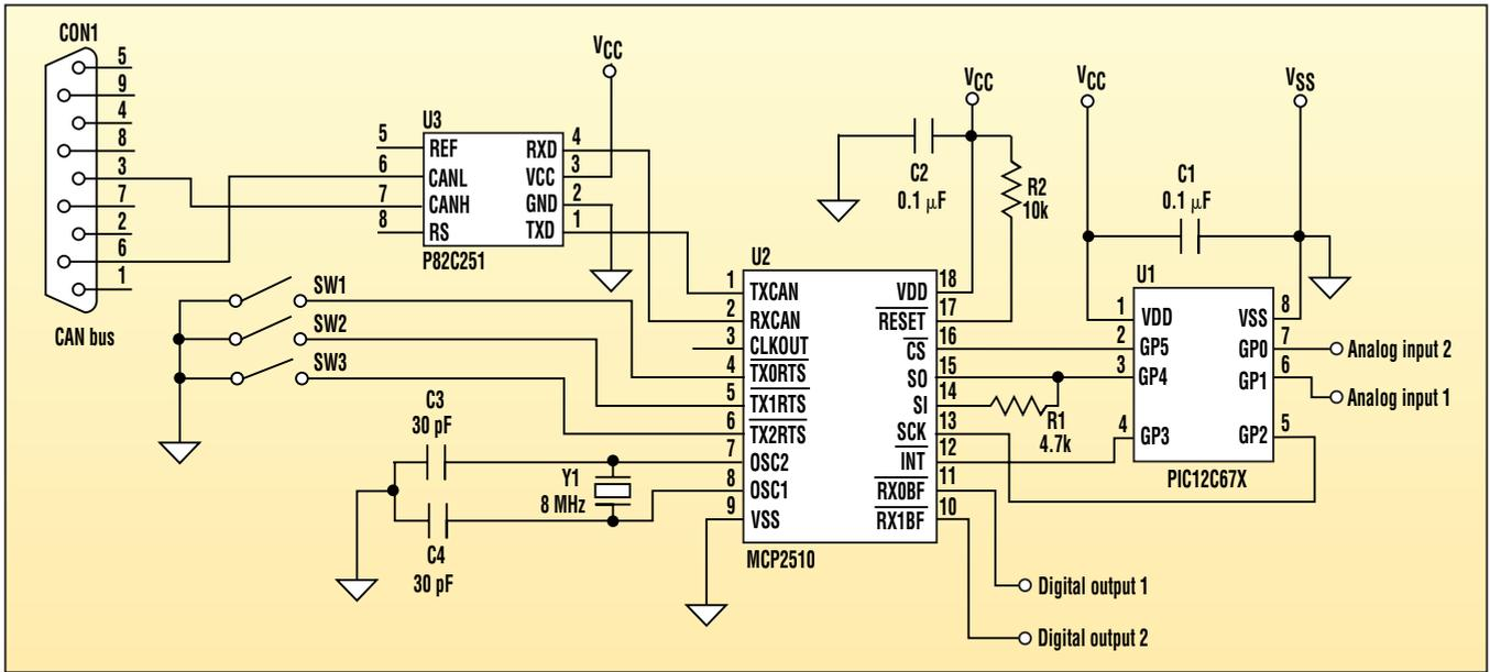
1. Using a diminutive 8-pin microcontroller, this CAN node provides two analog input channels and six digital I/O channels.
