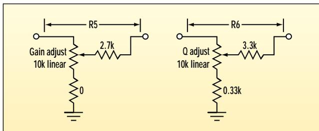
2. These networks can be substituted for R5 and R6 to provide variable gain and an adjustable Q value.
