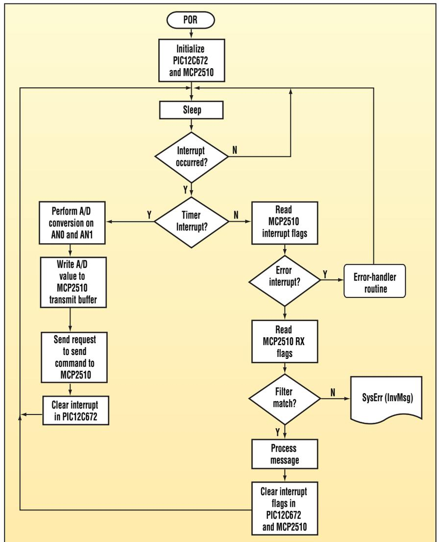
2. This CAN bus node provides both CAN-initiated and self-timed analog-to-digital conversions.
