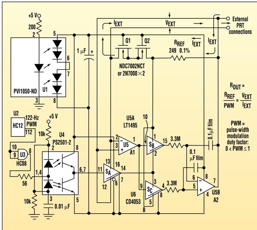
This DAC circuit simulates a 1000-Ω PRTD by outputting an optically isolated pure ohmic resistance in response to a PWM control input ( $R_O = R_{REF}/PWM$ ).
