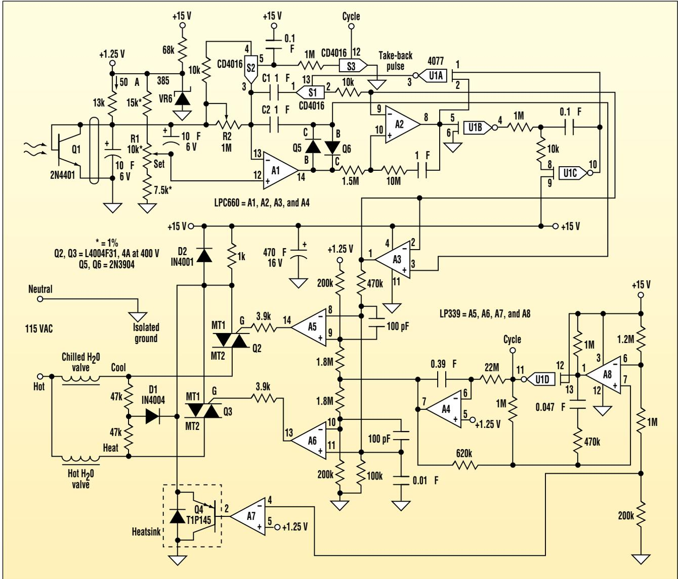
This TBH-based thermostat provides accurate and efficient environmental temperature control ( $\ll \pm 1^\circ\text{C}$ ), optimized with a single tuning variable.
