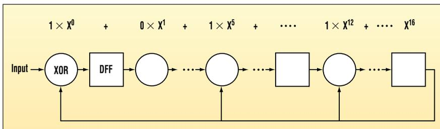
**The sample CRC-CCITT polynomial function of  $X^{16} + X^{12} + X^5 + 1$  can easily be generated for an Altera PLD by simply setting a few parameters in the AHDL code.**
