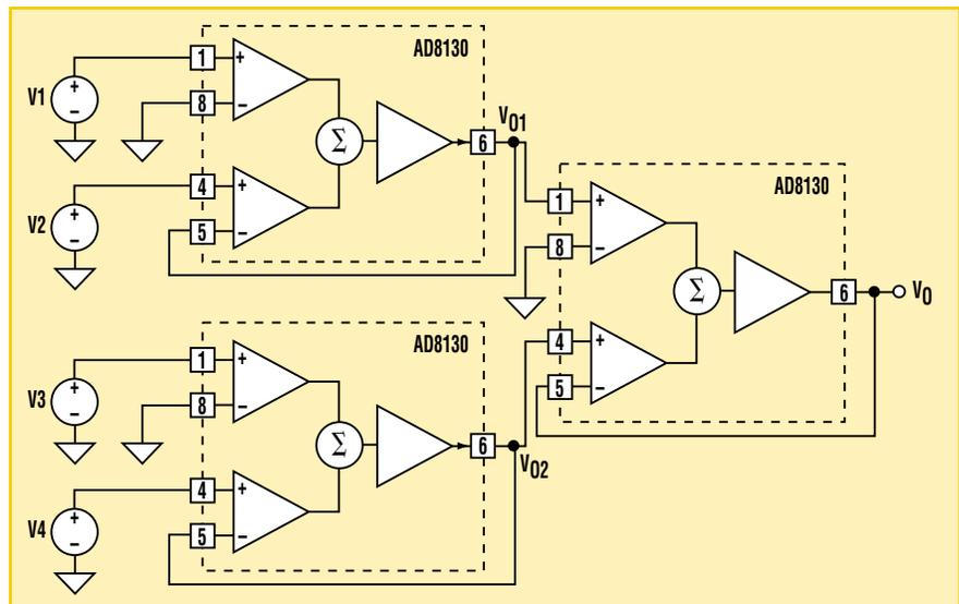
2. This high-speed summing amplifier can sum as many as four input voltages without the need for an inverter to change the sign of the output.
