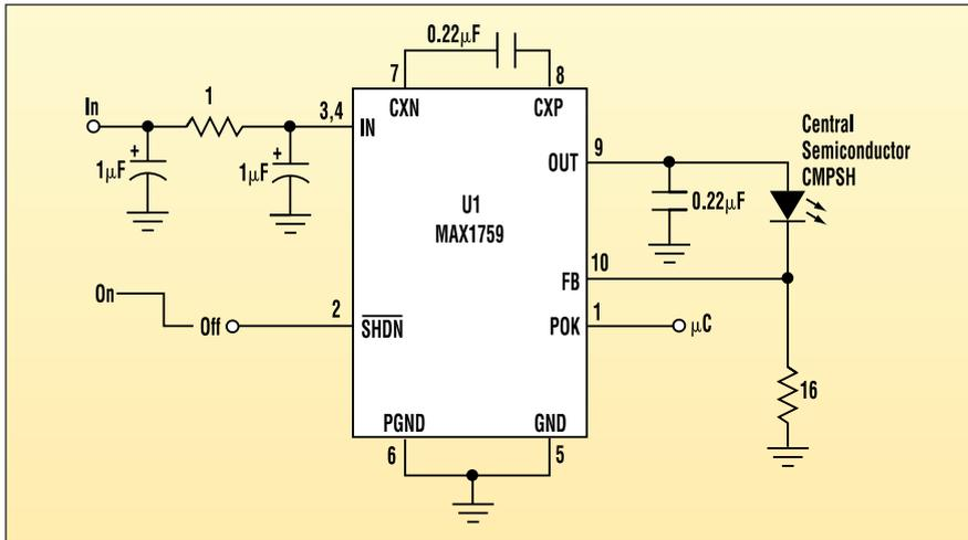
Unorthodox connections enable this charge-pump IC to directly regulate the current through a white LED backlight. The IC's shutdown feature prevents battery drain when the LED is off.
