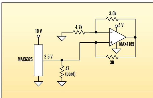
2. Placing the circuit from Figure 1 in parallel with the load of a voltage reference (47  $\Omega$  in this case) cancels most of the reference's resistive load. Effectively, only the capacitive load will
