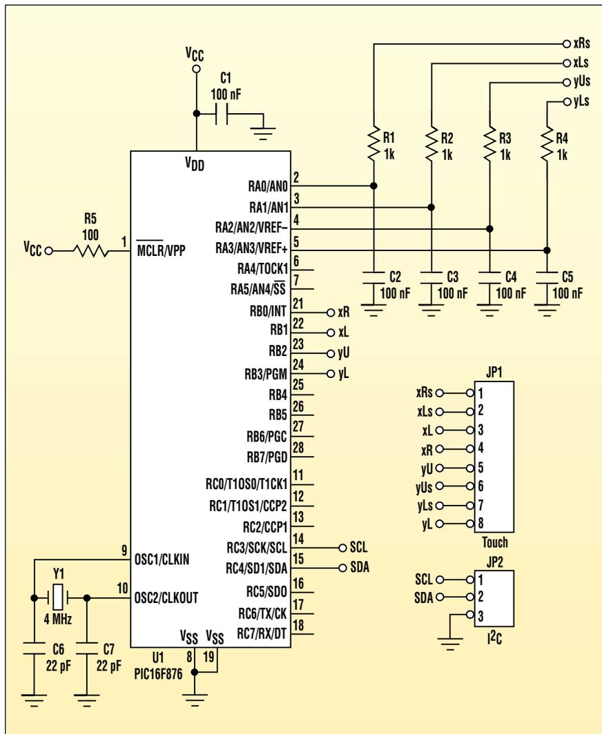
5. The PIC16F876-based eight-wire touchscreen controller includes a five-channel 10-bit ADC and supports the I<sup>2</sup>C interface. An optional low-pass filter has been added to eliminate noise.
