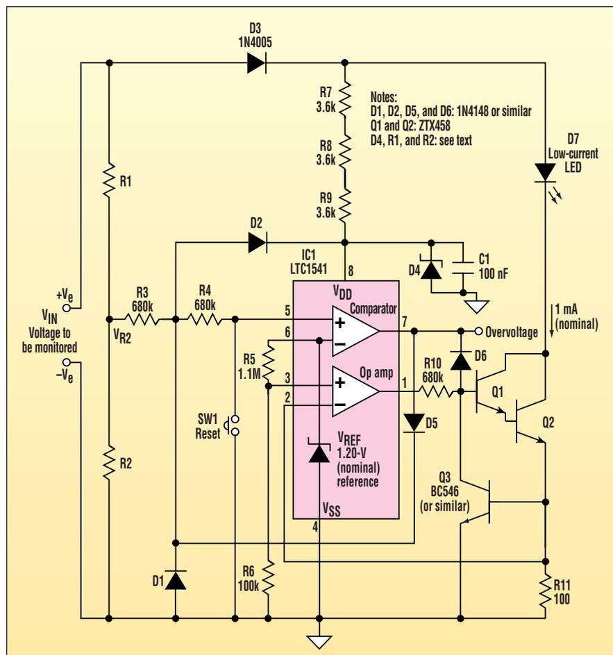
This latching overvoltage detector draws less than 25  $\mu$ A under normal operating conditions.
