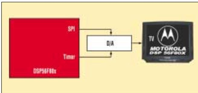
1. The on-screen display (OSD) combines a synchronization signal generated by an on-chip timer peripheral with the pixel-data signal output, also generated on-chip using an SPI peripheral.
