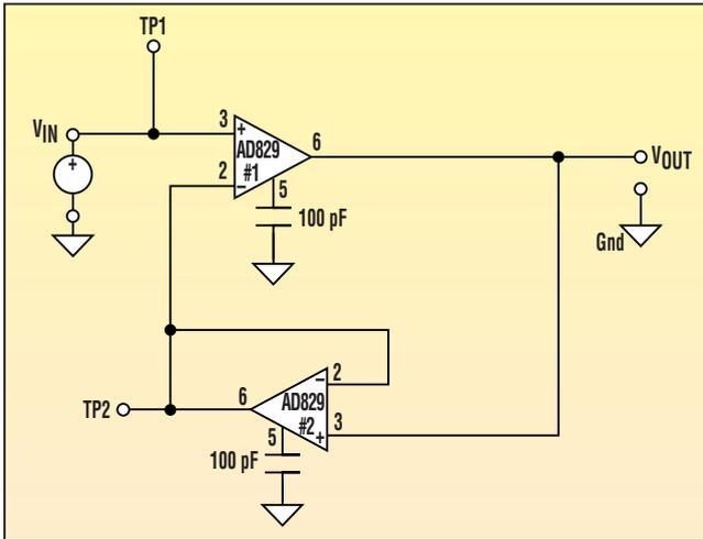
1. Adding an active feedback amplifier provides error cancellation, improving system error performance by as much as 20 dB.
