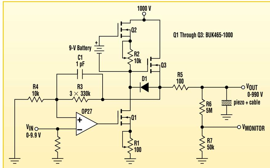
1. Rather than using piezo “stacks,” this low-cost 1-kV amplifier produces excellent results using less expensive “high-voltage” piezos, which are physically superior and easier to use.
