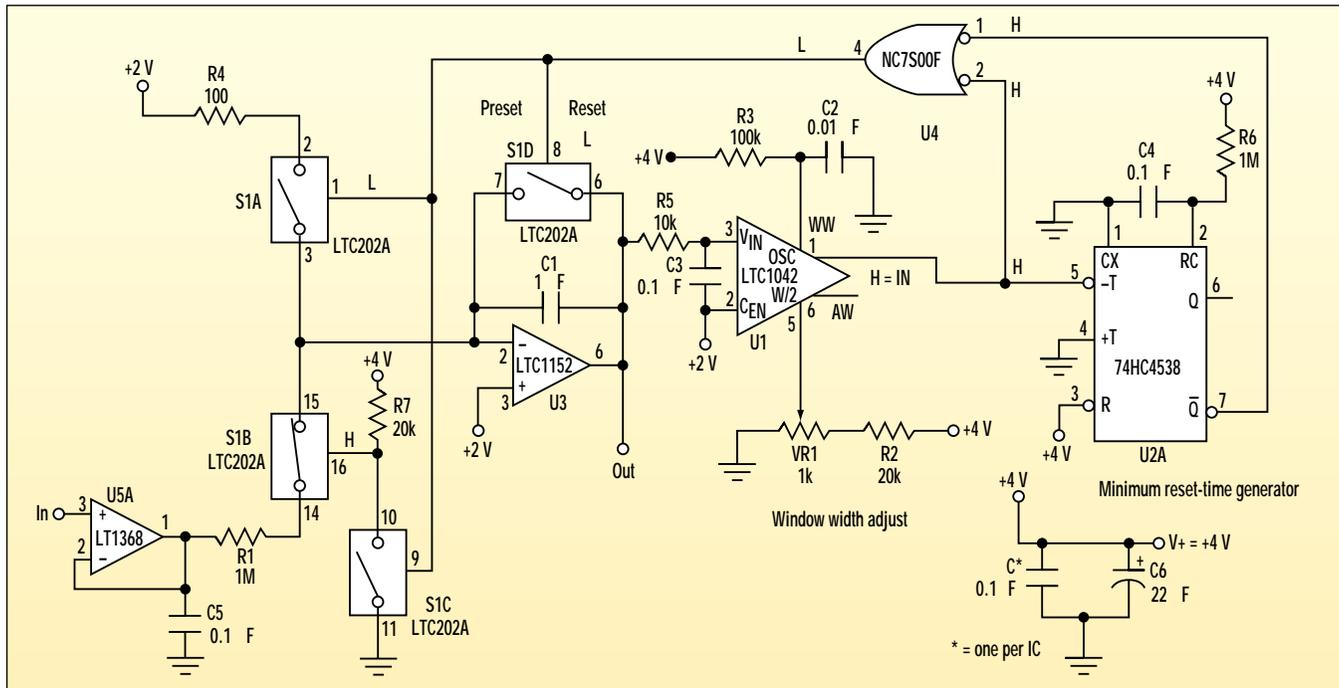
This easy to use window comparator building block is used to enhance performance and add intelligence to analog integrator circuits.
