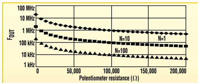
2. The output frequency for each divider value versus each tap location on the digital potentiometer is shown.
