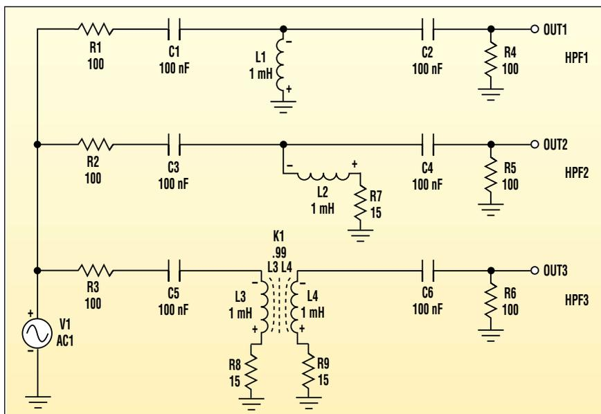
1. HPF1 is an ideal third-order high-pass filter with an ideal inductor. While HPF2 is the same filter with a non-ideal inductor, HPF3 replaces the inductor with a transformer.
