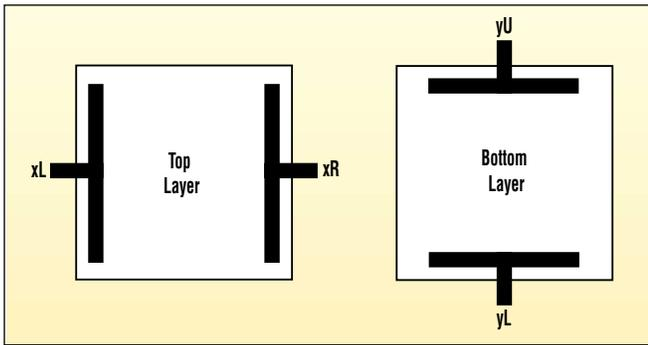
1. The four-wire touchscreen is decoded by placing a voltage across the top layer and reading the horizontal touch location on the bottom layer. The process is then reversed and a vertical touch location voltage is read from the top layer.
