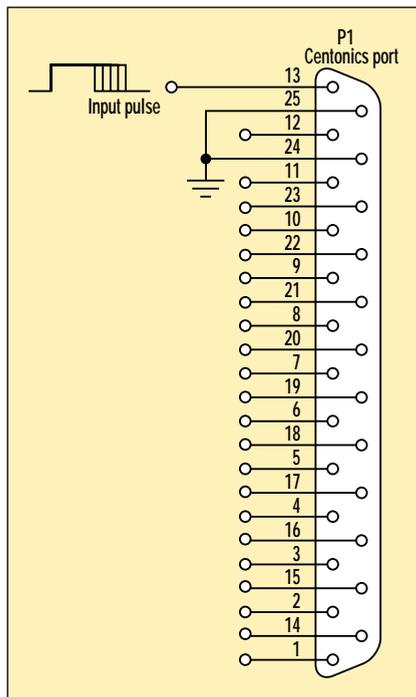
Single-wire sensors can be acquired directly by a PC if the counter/timer associated with the PC speaker function is reallocated for use by this application's pulse-width measurement function.
