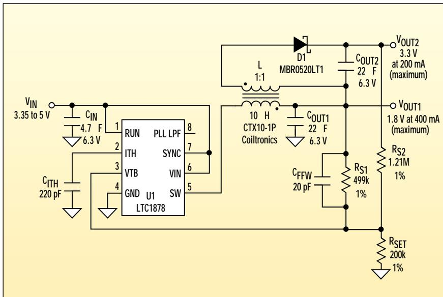
Implemented using an "overwinding" on the buck regulator's inductor, this circuit produces two quasi-regulated outputs by incorporating a dual-feedback arrangement.
