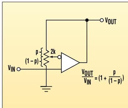
1. A decompensated op amp with the typical gain-set arrangement can exhibit instability when low gain settings are used.
