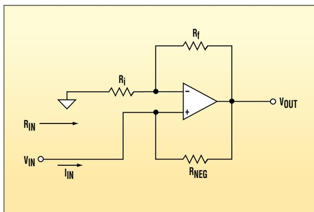
1. By matching this circuit's negative resistance (between the  $V_{IN}$  terminal and ground) with the load, the load will appear infinite.
