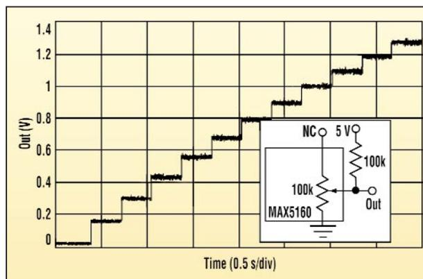
2. The resistance-ramp operation is observed by adding an external resistor to the wiper to form a voltage divider.
