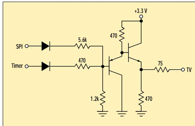
2. This simple circuitry converts the two digital signals into an analog-video signal and matches the 75- $\Omega$  input impedance of the TV set.
