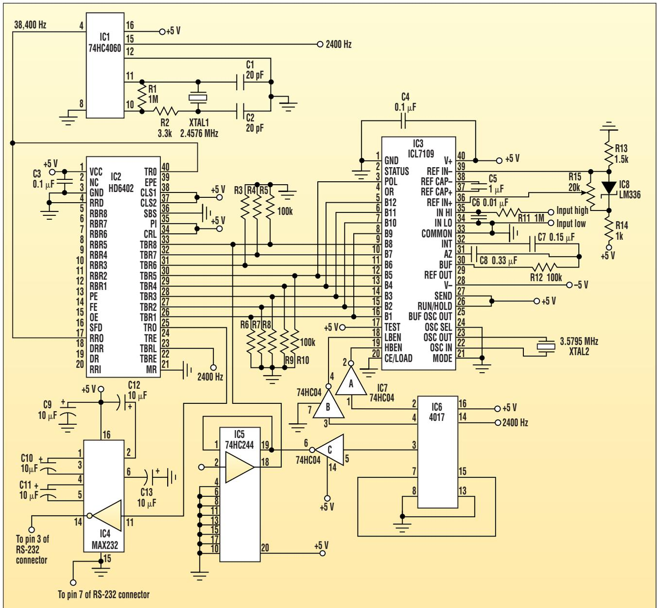
This low-cost 12-bit data acquisition system can be used to capture data from almost any external transducer and transfer it to a computer. The recorder, which connects to the computer's serial port, uses firmware that runs under either GWBasic or QBasic.
