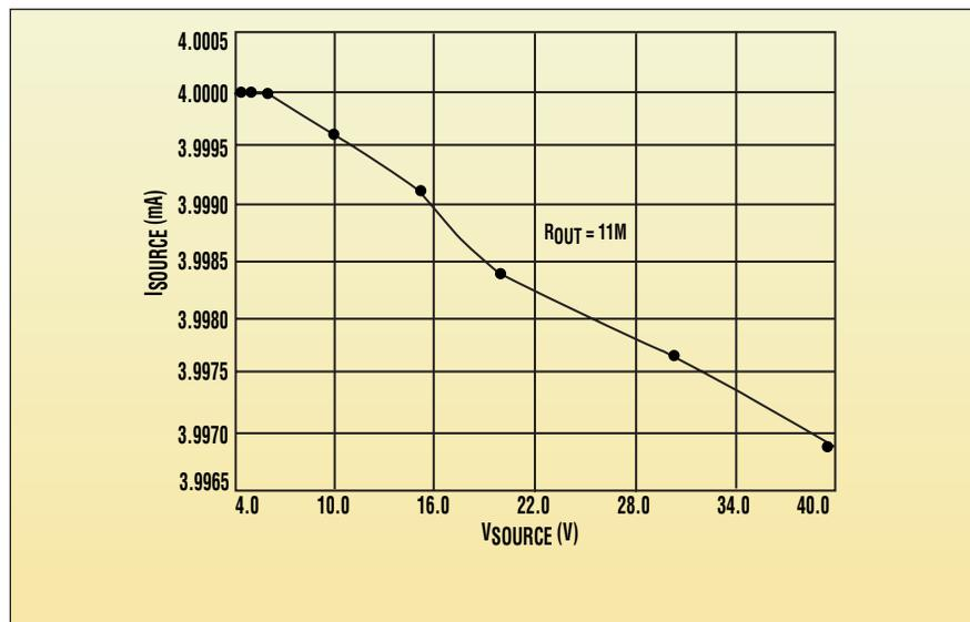
2. This plot of  $I_{SOURCE}$  versus  $V_{SOURCE}$  demonstrates that the composite op amp and voltage-reference current source has an output resistance of approximately 11 MΩ.
