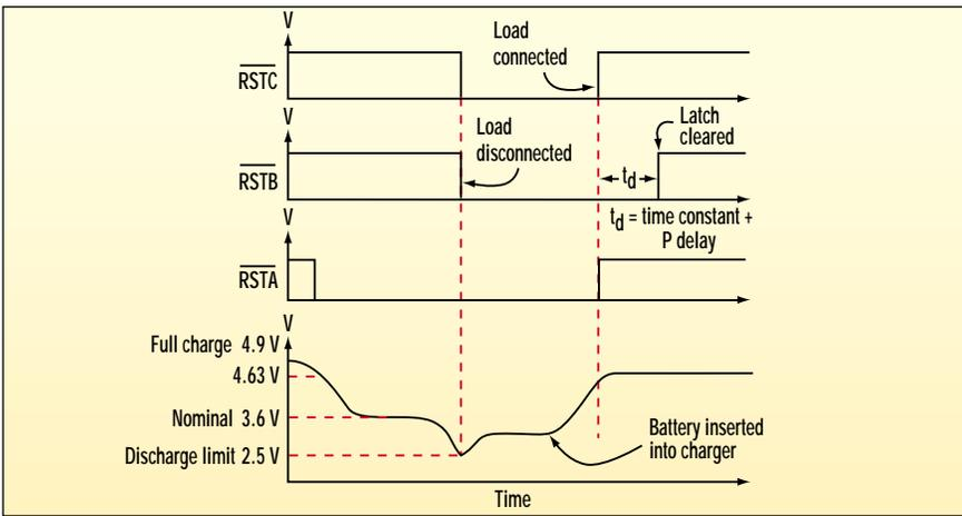
2. The response of the three reset signals in Figure 1 is shown over a typical discharge-charge cycle. The battery voltage profile is shown in the bottom waveform.
