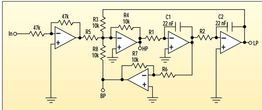
1. The building block of the basic filter provides low-pass, bandpass, and high-pass outputs.
