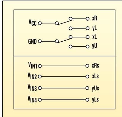
4. Designers can eliminate the need for multiplexing of the sense lines if a four-channel ADC is available in the system.
