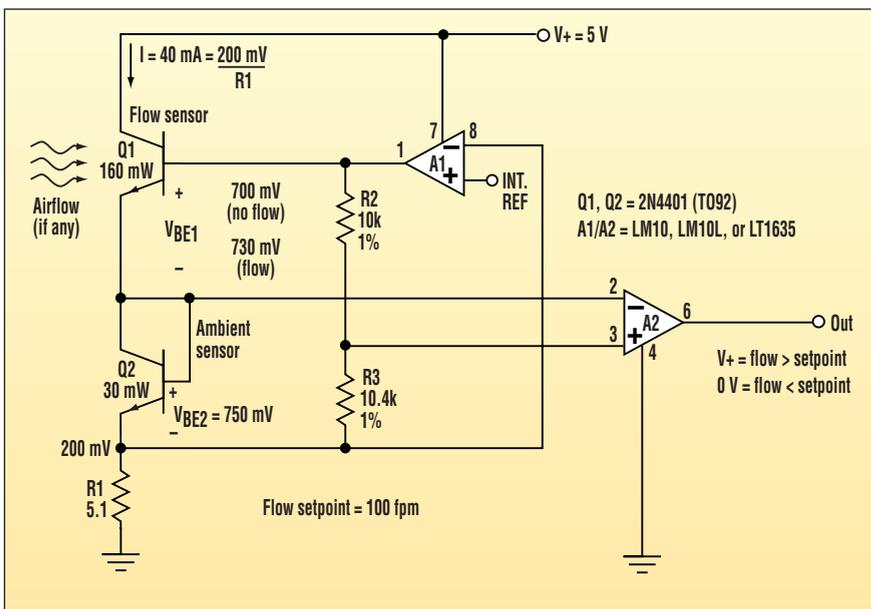
1. This airflow detector uses an ambient-compensated detection scheme based on differential heating of a series-connected transistor pair.
