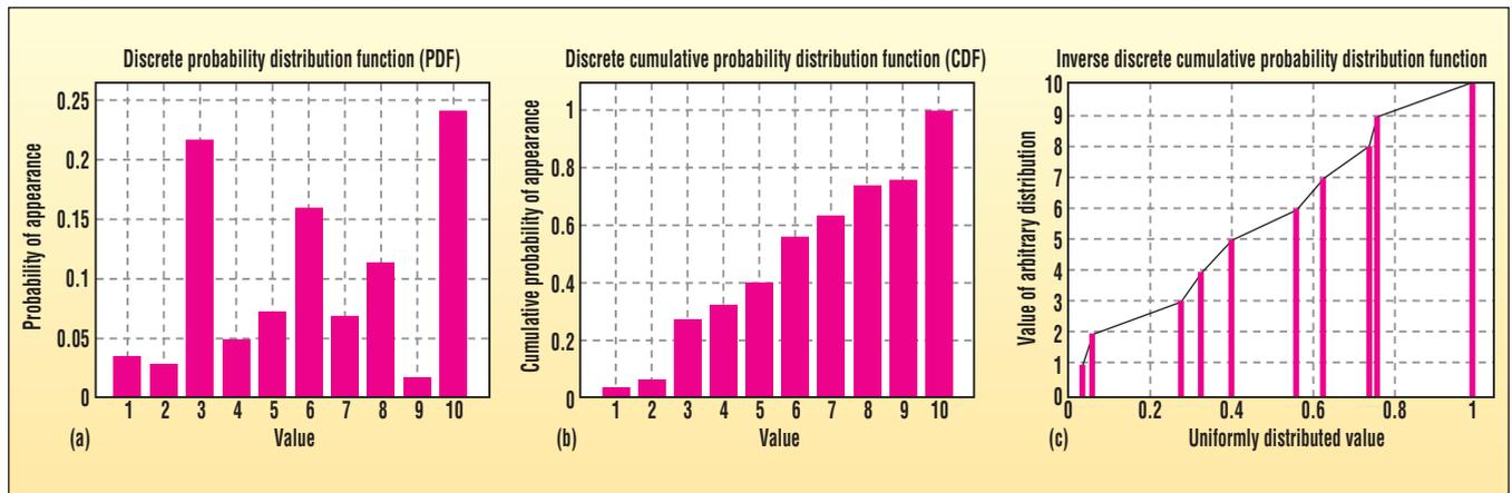
1. An arbitrary distribution is generated by analyzing the probability distribution function (a) and the cumulative distribution function (b) to create the inverse cumulative distribution function (c). The resulting CDF function is then embedded in the PROM contents.
