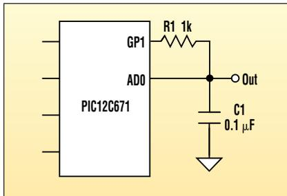
**1.** By taking advantage of the microcontroller's internal analog-to-digital (A/D) peripheral, an 8-bit digital-to-analog (D/A) output can be implemented with the addition of only a resistor and a capacitor.
