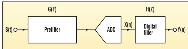
1. A typical DSP digital-filter channel incorporates an anti-aliasing prefilter prior to the analog-to-digital converter.
