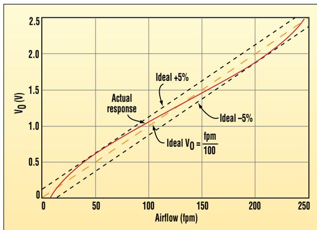
2. The quadratic relationship between  $I_Q$  and Q1/Q2's power dissipation does a fair job of canceling nonlinearity, erasing all but  $\pm 5\%$  FSR linearity error over the range of on-scale airspeeds.
