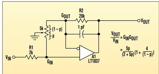
3. By modifying Figure 2b's topology, the input attenuator can be made variable by grounding the pot wiper to create two mechanically linked but electrically independent variable resistors.
