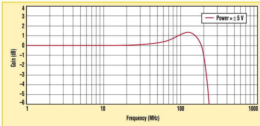
4. The bandwidth of the improved summing amplifier is about 220 MHz.
