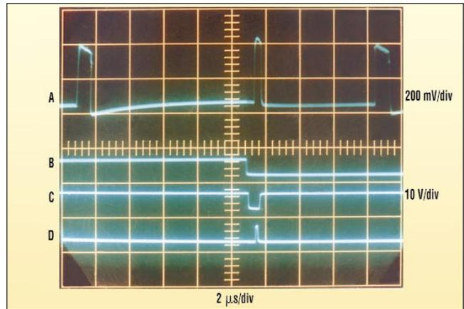
2. The input signal V<sub>IN</sub>, trace A, is intensity-modulated by the MAX997 output, trace B. Trace C shows one of the MAX961 T/H driver outputs. The delay-qualified trigger, trace D, is exclusively synchronized to the central, narrow pulse at V<sub>IN</sub>.
