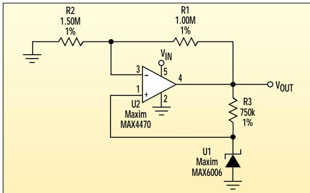
A shunt reference (U1) in this series-reference circuit yields a composite circuit that provides the low power consumption of a shunt reference with the line-load regulation of a series reference.
