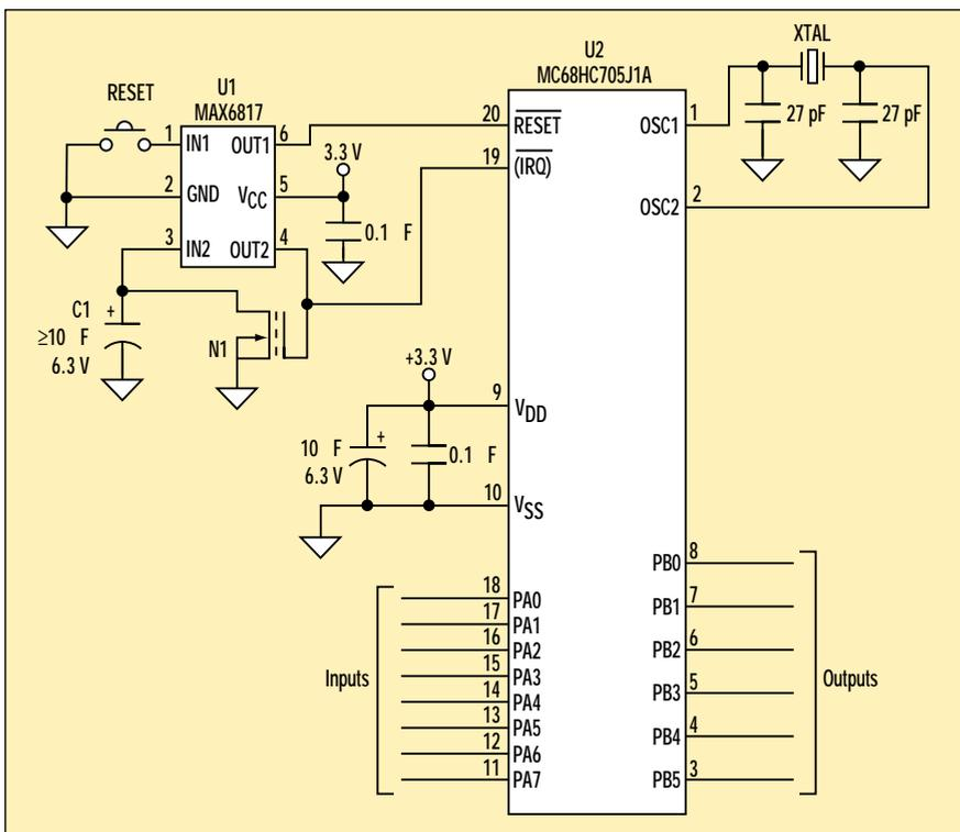
In addition to debouncing the microcontroller's RESET input, the unused half of this dual switch-debouncer IC (U1) is used to implement a long-period timer function.
