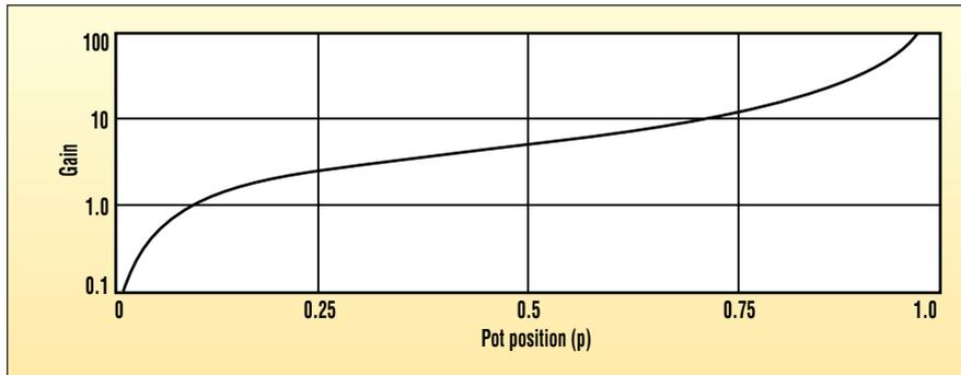
4. The resulting composite gain-versus-p curve ( $G = G_1 \times G_0$ ) is shown. The possible gain settings extend from zero (at  $p = 0$ ) to the open-loop gain of the op amp (at  $p = 1$ ).
