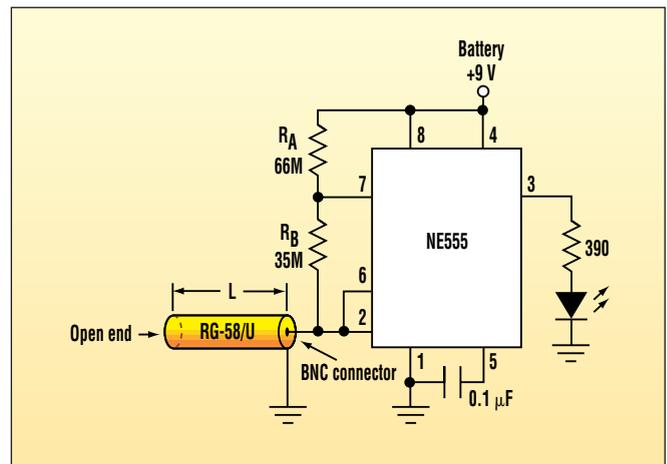
A simple and inexpensive “reflectometer” locates cable breaks using the distributed cable capacitance and ratiometric calculations.
