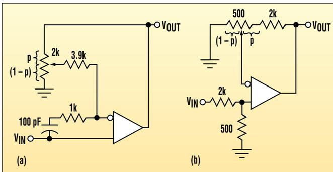
2. Overcoming the  $G_{MIN}$  problem can be accomplished using an ac-gain-limiting network (a) or a brute-force  $1/G_{MIN}$  input attenuator (b).
