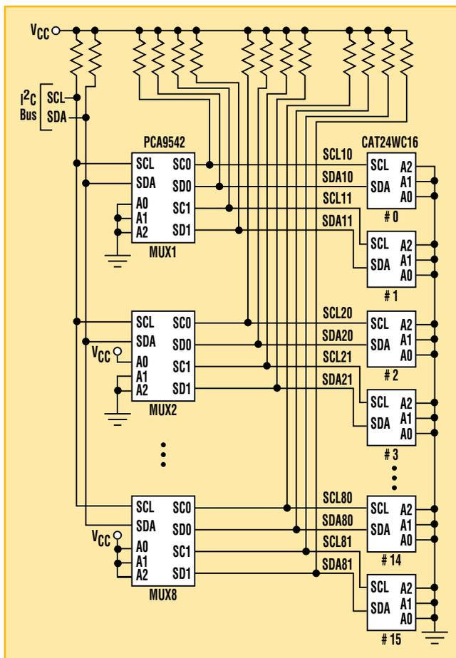
Multiple non-I<sup>2</sup>C-addressable serial devices, like these CAT24W16 serial EEPROMs, can be interfaced to the I<sup>2</sup>C bus using Philips PCA9542 I<sup>2</sup>C multiplexers.
