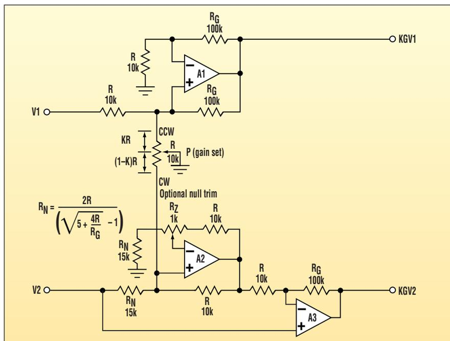
Instead of using a ganged pot, grounding the wiper terminal of a single pot creates two mechanically linked but electrically independent variable resistances: KR and (1-K)R.
