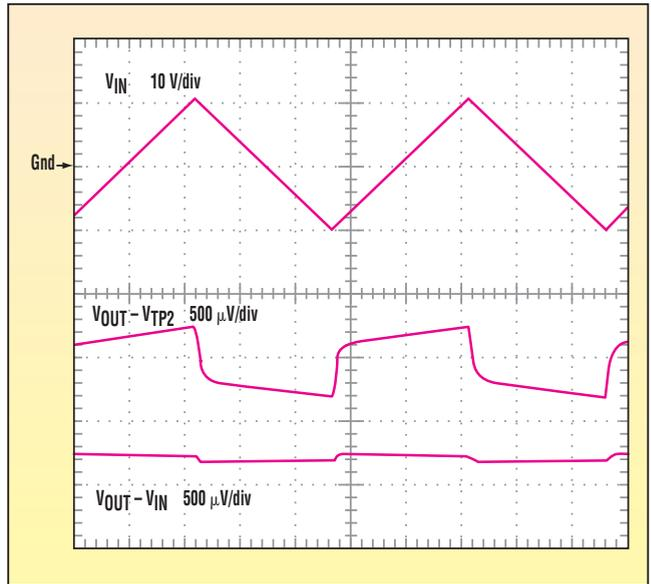
3. The performance of this circuit using a ±10-V triangle waveform input at 1 kHz indicates error reductions similar to those in Fig. 2.
