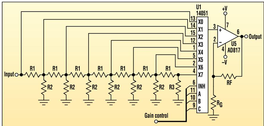
This wide-bandwidth, low-distortion programmable gain amplifier (PGA) is built using low-cost standard devices, eliminating the need for an expensive programmable-gain amp IC.
