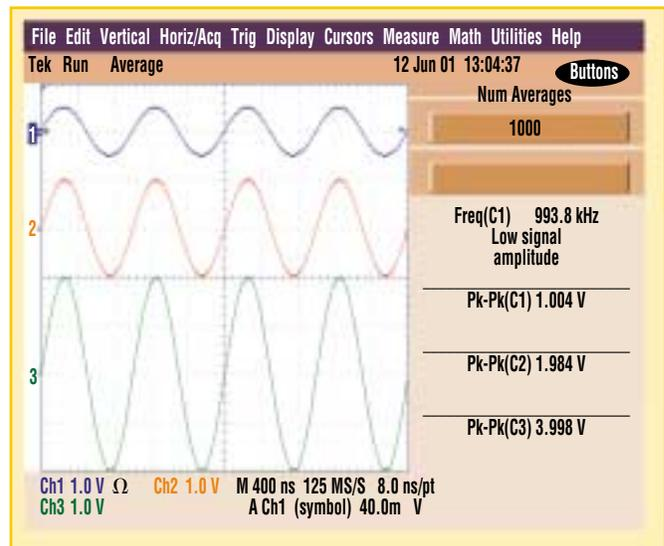
3. The performance of the high-speed summing amp at 1 MHz is shown. The top trace is the input signal for all four inputs. The middle trace is the sum of inputs V1 and V2. The bottom trace is the summing output.
