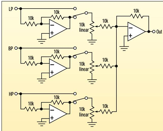
4. This linear-combination arrangement can be used to provide several different types of useful filter characteristics.
