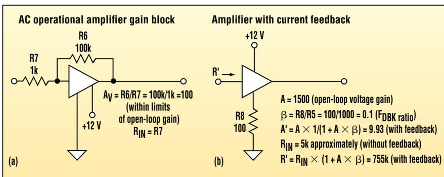
2. The circuit may be redrawn as an op-amp gain block with external components controlling the gain (a). An alternative hookup uses a resistor in the ground-return circuit (b).
