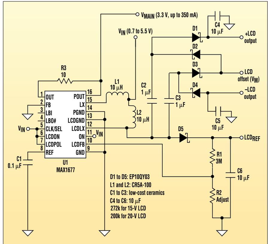
2. Implemented using a high-efficiency, dual-output boost converter, this single-IC circuit generates the dual voltages that are required to control the contrast in an STN LCD.
