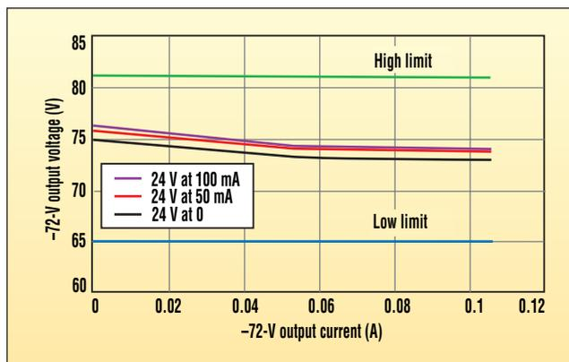
**2. The load regulation of the -72-V output is well within the  $\pm 14$ -V telephony requirements. The worst-case variation is less than 4 V.**
