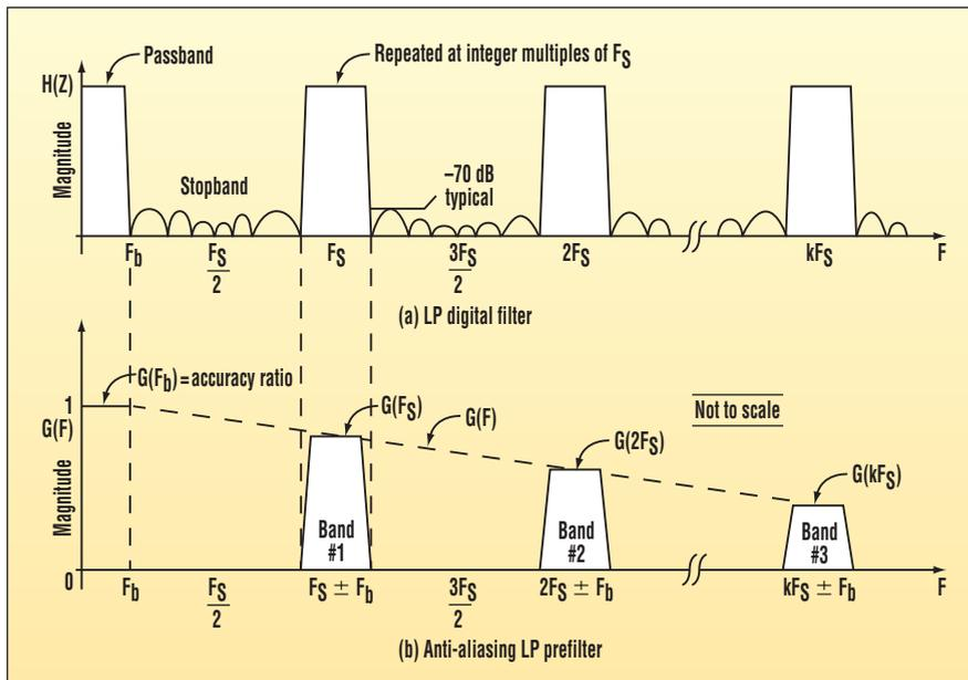
**2.** A low-pass digital filter (a) attenuates the spectra in the stopbands and passes the spectra in the passbands ( $kF_s \pm F_b$ ) which are aliased to the band of interest ( $0 - F_b$ ). Use of the prefilter (b) constrains the aliasing within the required limits.
