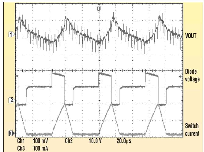
2. Unstable duty cycles cause a higher quiescent current, larger current peaks, and a bigger output ripple. The duty cycle alternates from one cycle at 75% to two cycles at 0%.
