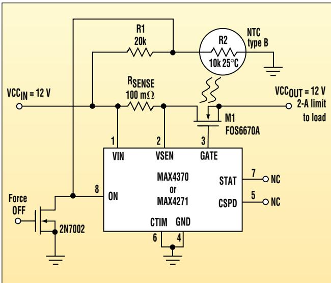
1. Combining a few components with a hot-swap controller IC yields a precision current-limited supply for 3- to 12-V loads.
