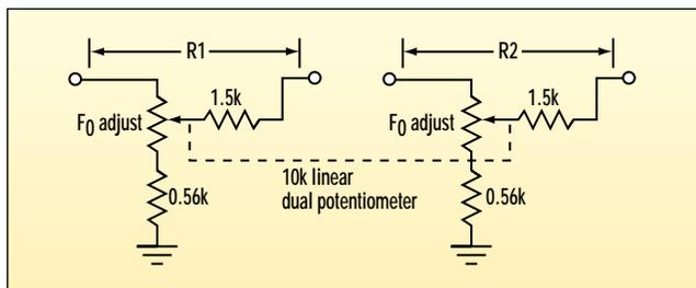
3. If variable adjustment of characteristic frequency,  $f_0$ , is required, these networks can be substituted for R1 and R2.
