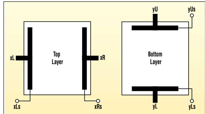
2. An eight-wire resistive touchscreen is similar to the four-wire version. It has four additional sense lines to improve accuracy and counter environmental effects.
