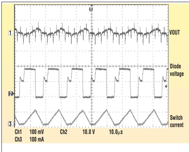
1. A dc-dc converter designed to maintain a constant 45% duty cycle produces a lower quiescent current and lower output ripple..
