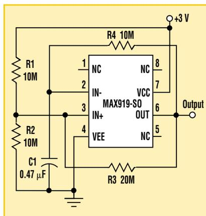
The use of an oscillator based on an ultra-low-power comparator can provide significant battery-life improvements.
