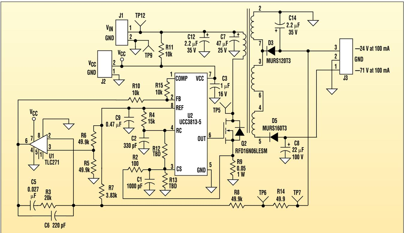
1. This multi-winding flyback power supply allows a single control circuit to regulate both voltage outputs.
