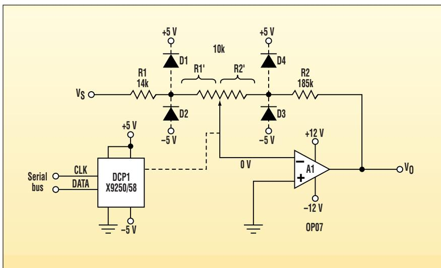
This amplifier's virtual ground allows the  $\pm 12$ -V circuit shown to use a  $\pm 5$ -V digital pot for gain control. Due to the need for a virtual ground, noninverting configurations can't be used.
