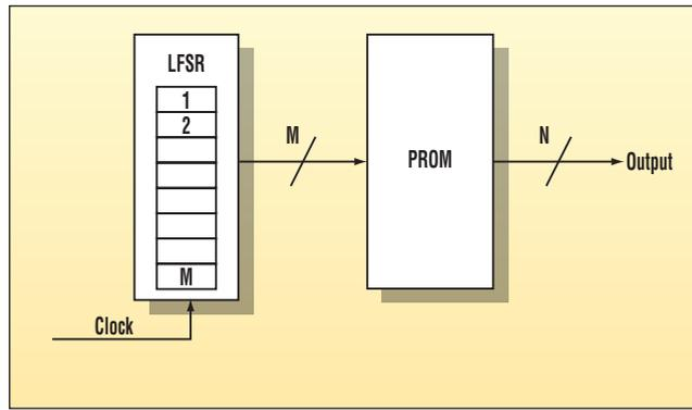
2. The high-speed hardware implementation of this random number generator allows the arbitrary output distribution to be controlled by the inverse cumulative distribution function.
