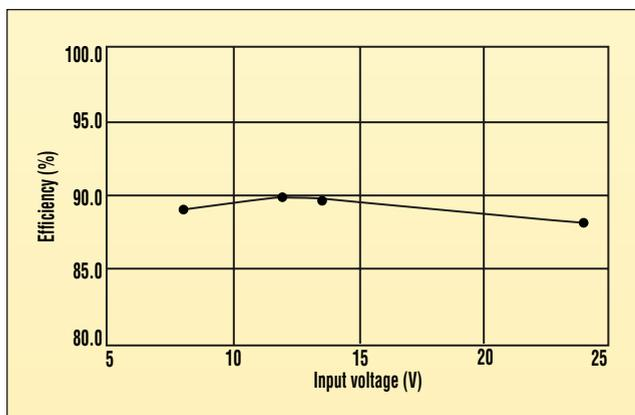
**3. The low conduction and switching losses of the n-channel MOSFET help to provide excellent efficiency performance.**
