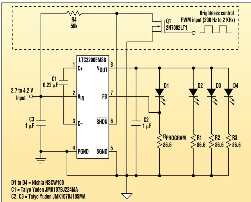
With this inductorless step-up circuit, constant-current output control drives white LEDs regardless of the magnitude or variations in their forward-voltage characteristics.
