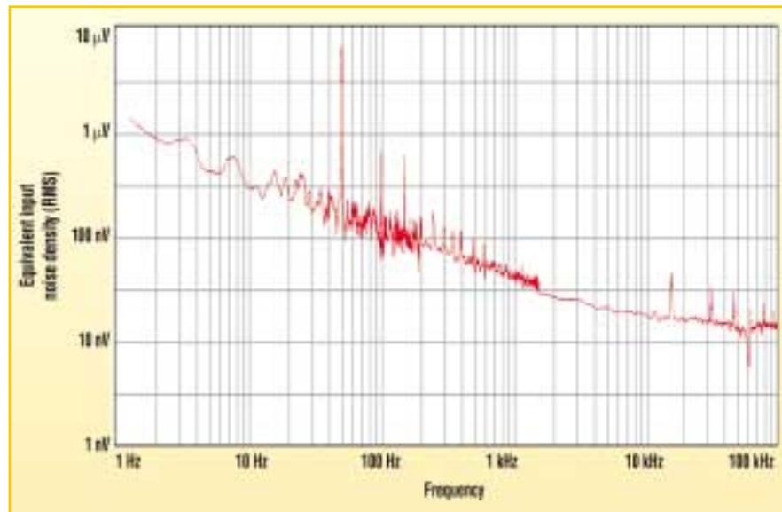
2. The equivalent input noise density of the amplifier versus frequency is shown.
