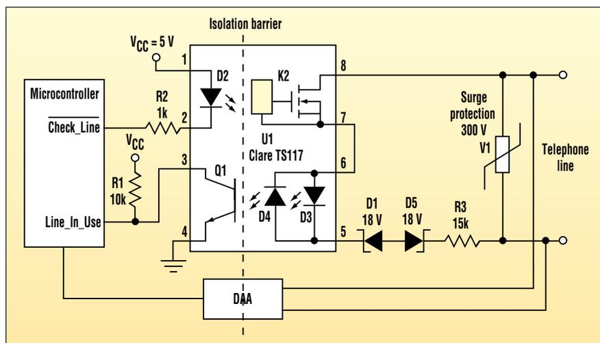
Using a solid-state optoisolated relay to apply a voltage detector to the phone line helps this detector circuit meet the FCC requirements for on-hook impedance limits.
