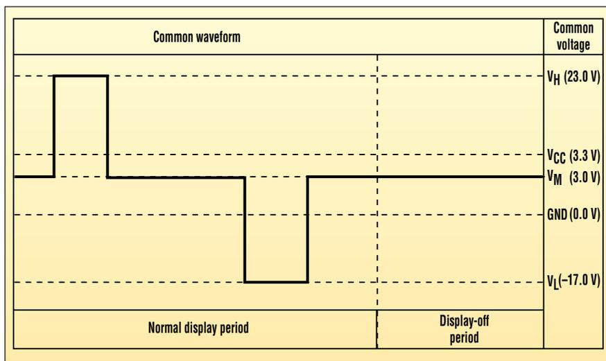
1. In order to avoid creating a damaging dc component across the LCD, the contrast waveforms generated by the supply must be symmetric about the LCD reference level  $V_M$ .
