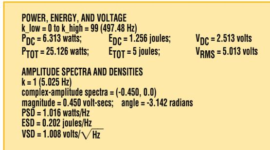
2. The DFT results of the sample pulse waveform in Figure 1 are shown.
