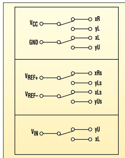
3. When multiplexing sense lines for an eight-wire touchscreen, the sense lines are individually multiplexed to the inputs of the microcontroller's five-channel ADC.
