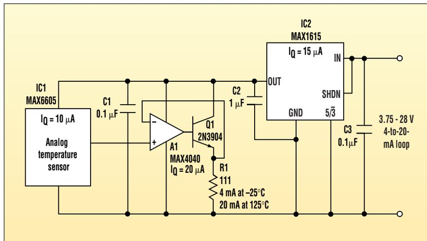
Using low-quiescent-current devices, this temperature sensor derives its power directly from the 4-to-20-mA current loop. This results in a slight offset error that can be compensated out.
