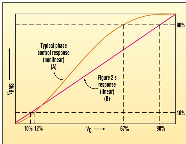
**1. A typical thyristor phase-control response (plot A) compresses 80% of the thyristor rms output range in 55% of the control-input range. A circuit using a control-voltage-to-trigger angle converter produces both adequate gain and non-oscillatory stability (plot B).**
