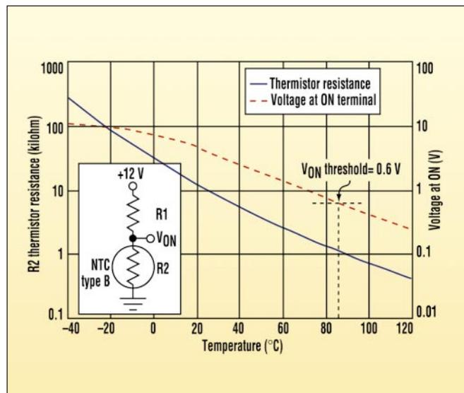
2. The NTC thermistor resistance variation with temperature is shown. A thermal cutoff threshold of 85°C results.
