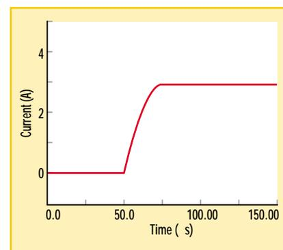
4. During a successful fuse reset, the current rises to its normal operating level in 25  $\mu$ s.
