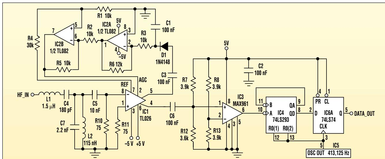
This noncoherent, narrowband FSK receiver doesn't employ any PLLs, high-quality-factor bandpass filters, or trimming adjustments.
