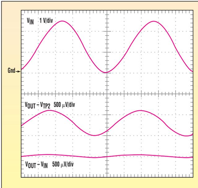
2. With this amplifier, using a 0- to 2.5-V 10-kHz sinewave input, a significant error reduction is seen when the buffer amp error (middle trace) is compared with the output error (bottom trace).
