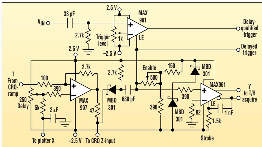
1. A 250-Ω control sets the delay of the MAX997's step pulse to modulate the CRO beam, trigger the strobe and the T/H for the X-Y plotter, and enable the delay-qualified trigger.
