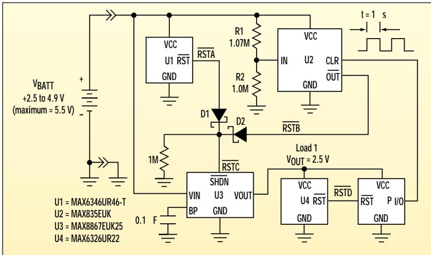
1. This micropower circuit provides shutdown, power-up, and low-battery lockout functions for this three-cell NiCd-based circuit without the need for software or operator control.
