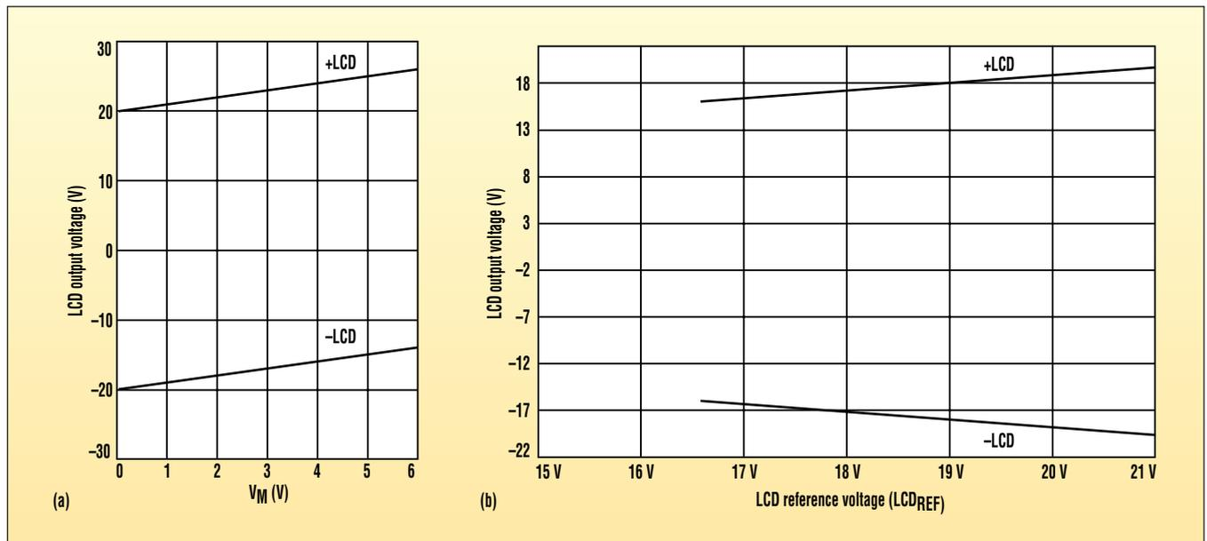
3. The  $\pm\text{LCD}$  outputs track each other and the LCD reference voltage (a), as well as the sum of V<sub>M</sub>  $\pm$  LCD<sub>REF</sub> (b).
