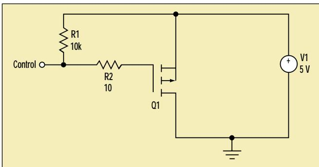
1. This heater circuit utilizes the fact that FETs designed for high-voltage switching applications often feature high  $R_{DS(ON)}$  values.
