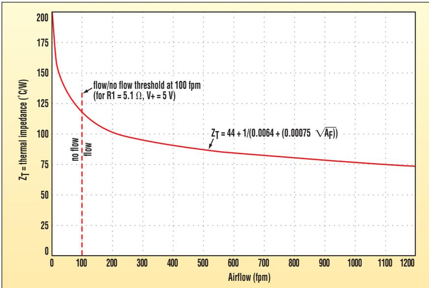
**2. The TO-92 packaging of the sensor selected has a thermal-impedance-versus-airspeed characteristic that is well approximated by a simple equation.**
