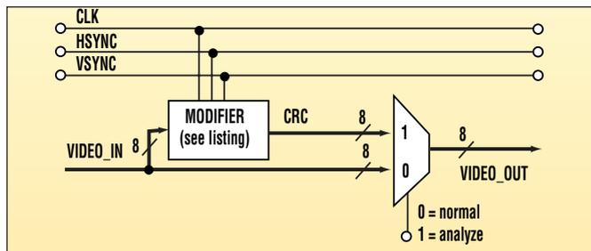
The video modifier replaces the normal video signal with a CRC-based signal to visually exaggerate errors on the video display itself. One of the three video channels (red, blue, and green) is shown.
