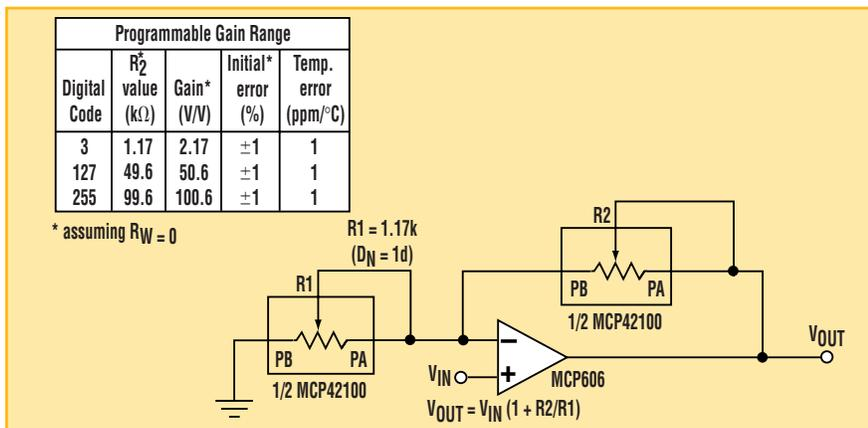
3. The intrinsic matching of a dual digital pot is used to achieve an initial gain accuracy of ±1% (max.) and a typical temperature coefficient of 1 ppm/°C.
