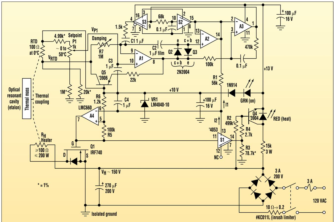
In addition to the "Take-Back-Half" control algorithm (TBH), this precision heating controller uses feed-forward compensation to virtually eliminate the effects of sudden ac-line variations. The sampling of the heater supply voltage ( $V_H$ ) is performed by S1 and the R2/R4 network.
