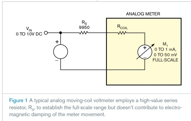
**Figure 1** A typical analog moving-coil voltmeter employs a high-value series resistor,  $R_S$ , to establish the full-scale range but doesn't contribute to electromagnetic damping of the meter movement.
