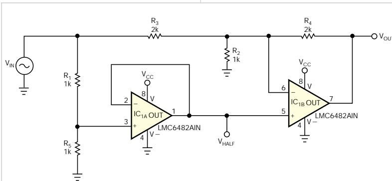
**Figure 1** This precision full-wave-rectifier circuit uses two op amps and no diodes. When altering the basic design, note that resistors  $R_3$  and  $R_4$  are both twice the value of  $R_2$  and that  $R_1$  and  $R_5$  are equal.
