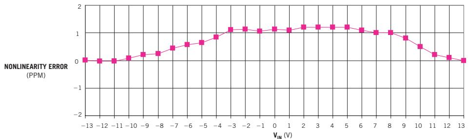
The circuit in Figure 2 introduces a maximum nonlinearity error of about 1 ppm over a 26V input-voltage range.
