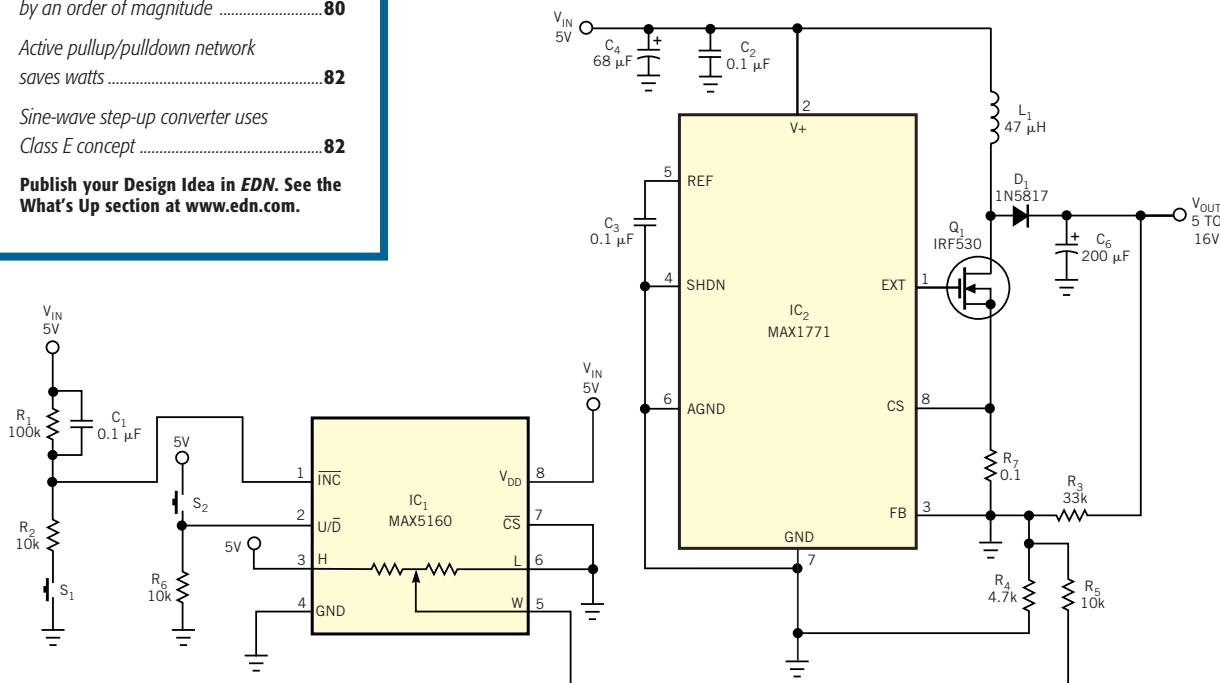
A digital potentiometer, IC<sub>1</sub>, and two pushbutton switches, S<sub>1</sub> and S<sub>2</sub>, let you adjust the regulated output voltage of boost converter IC<sub>2</sub> over a 10V range.
