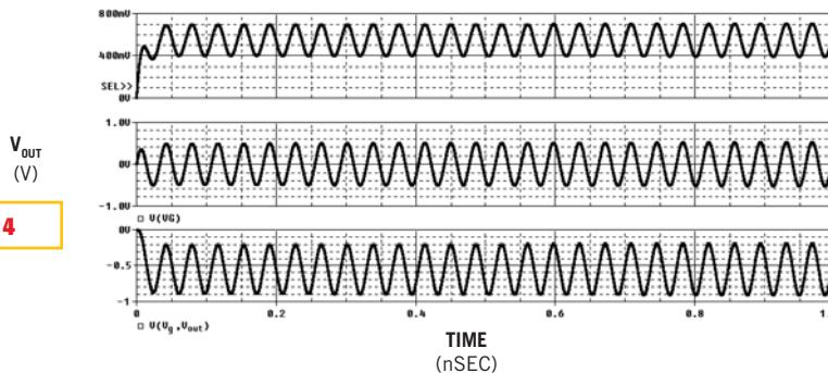
With  $C_1$  having a value of 50 nF and  $C_2$  having a value of 114 nF, the circuit oscillates.
