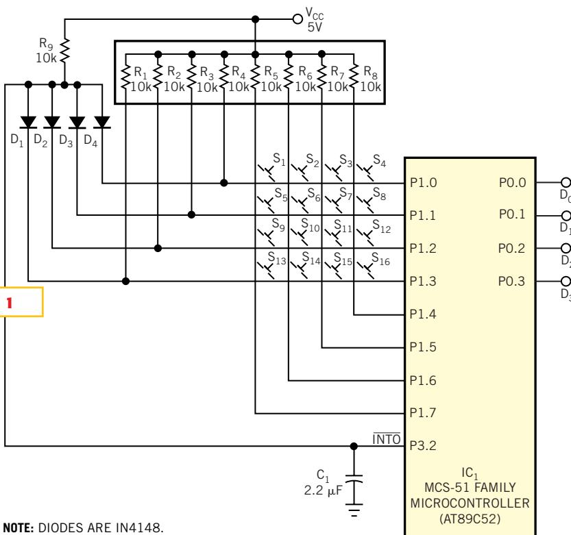
**Adding an interrupt-driven keypad to an MCS-51 family microcontroller requires only a few components.**
