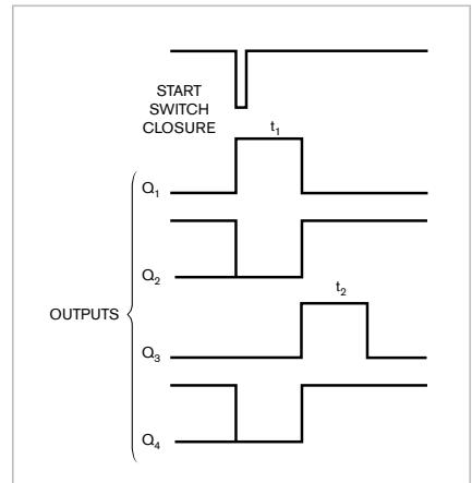
**Figure 2** This timing diagram illustrates outputs available from the timer's two sections.
