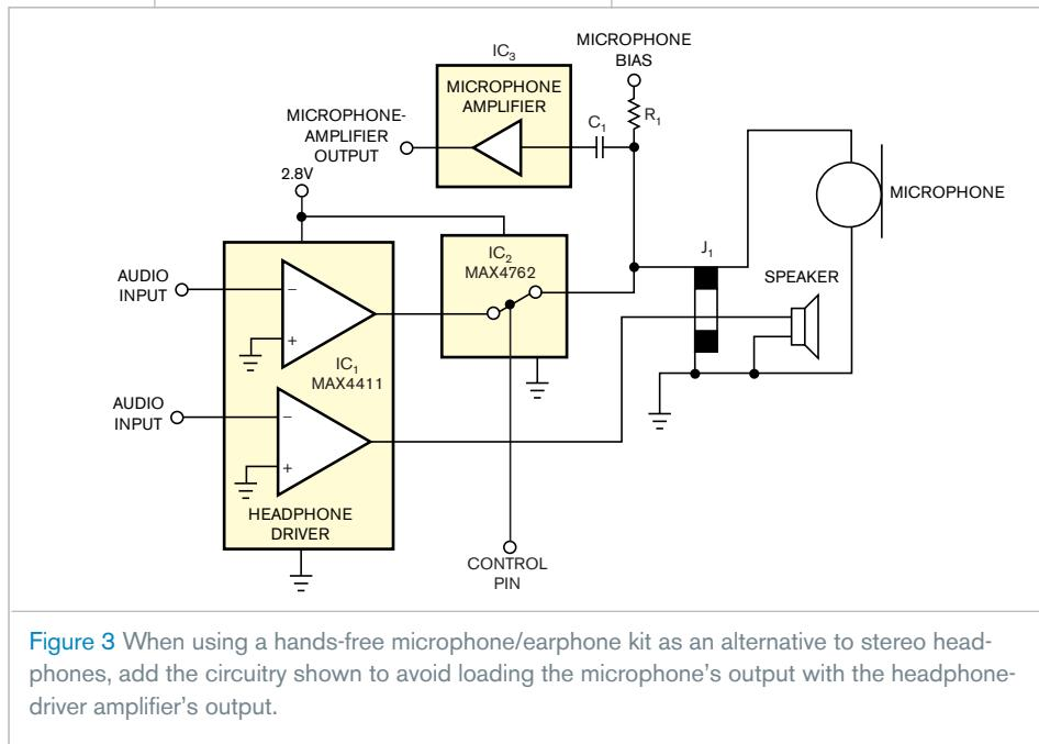
Figure 3 When using a hands-free microphone/earphone kit as an alternative to stereo headphones, add the circuitry shown to avoid loading the microphone's output with the headphone-driver amplifier's output.
