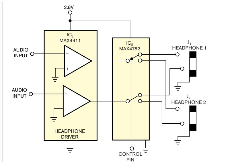
**Figure 1** For low values of power-supply voltage, 2.8V maximum, use an analog switch at IC<sub>2</sub> that handles signal amplitudes to  $V_{DD} - 5.5V$  to direct IC<sub>1</sub>'s bipolar outputs to the headphone loads.
