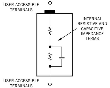
**Figure 1** An elementary model of a battery's internal impedance includes resistive and capacitive elements, but the capacitive elements introduce errors in ac-based impedance measurements. For improved accuracy, analyze the battery's voltage drop at a frequency near dc.
