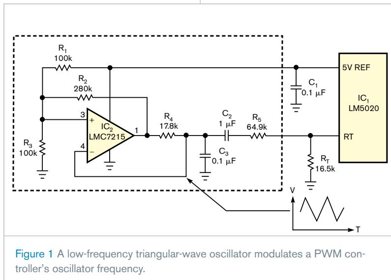
Figure 1 A low-frequency triangular-wave oscillator modulates a PWM controller's oscillator frequency.
