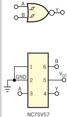
Connecting pins 1 and 2 to ground configures the NC7SV57 as a two-input NOR gate.
