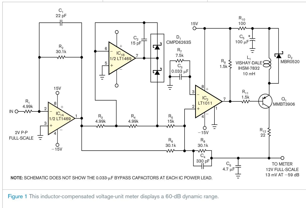
Figure 1 This inductor-compensated voltage-unit meter displays a 60-dB dynamic range.
