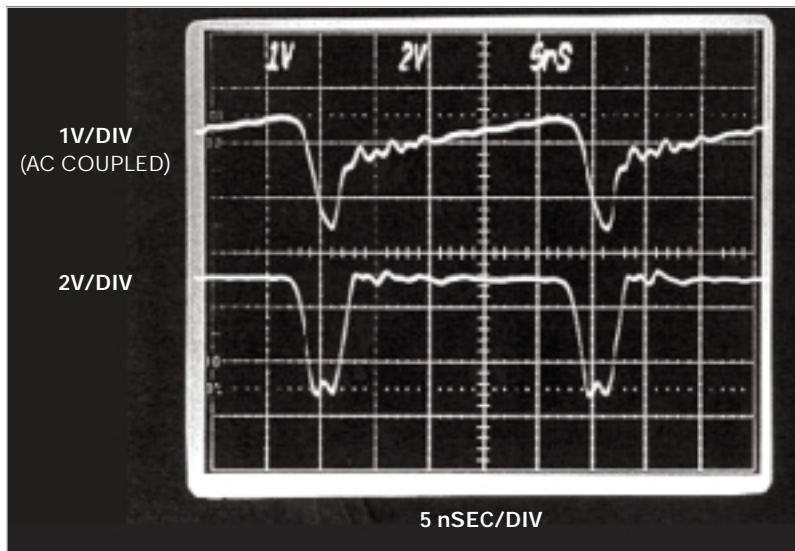
**Figure 2** On a 700-MHz real-time oscilloscope, the oscillator-core waveforms at a 40-MHz operating frequency show the ramp-and-reset waveform at Q<sub>1</sub>'s collector (upper trace) and Q<sub>2</sub>'s emitter (lower trace).
