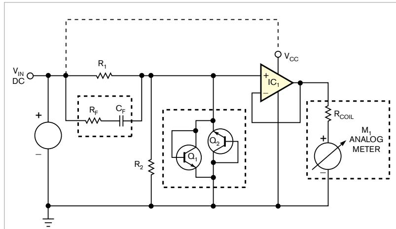
**Figure 2** An operational amplifier's low output resistance provides electro-mechanical damping for a moving-coil meter for stable readings and enhanced resistance to mechanical shock and vibration. Connect  $V_{CC}$  to either an external power supply or the circuit's input terminal if  $V_{IN}$  exceeds  $IC_1$ 's minimum power-supply-voltage rating.
