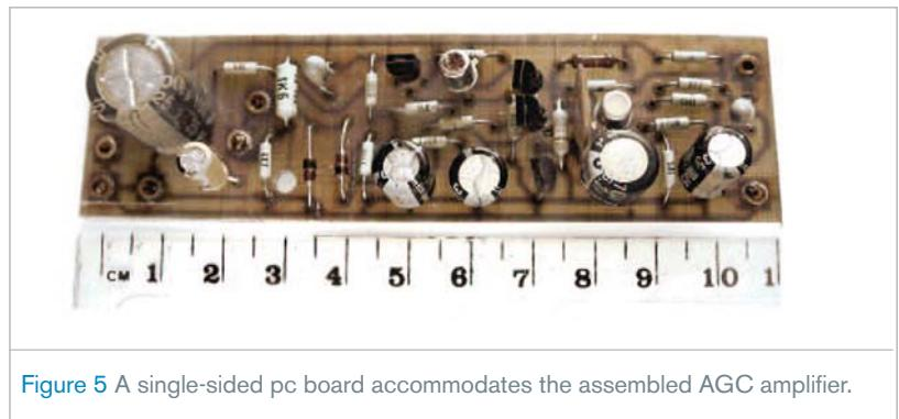
**Figure 5** A single-sided pc board accommodates the assembled AGC amplifier.
