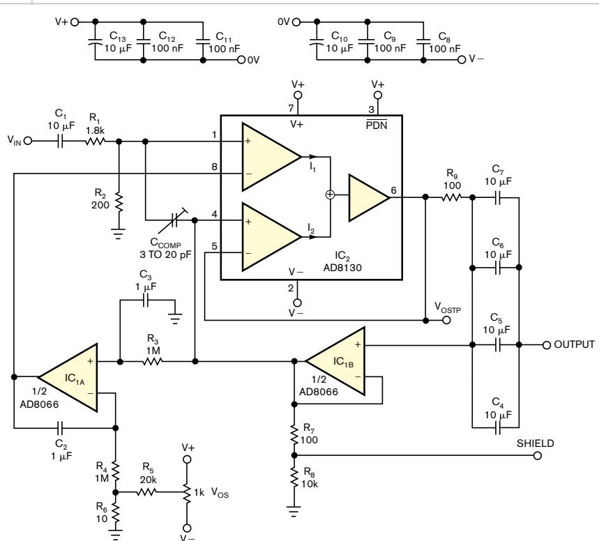
**Figure 4** The complete circuit includes trimmer capacitor C<sub>COMP</sub>, which compensates for stray capacitances in the circuit's packaged layout. Also, note wideband treatment of power-supply bypass capacitors.
