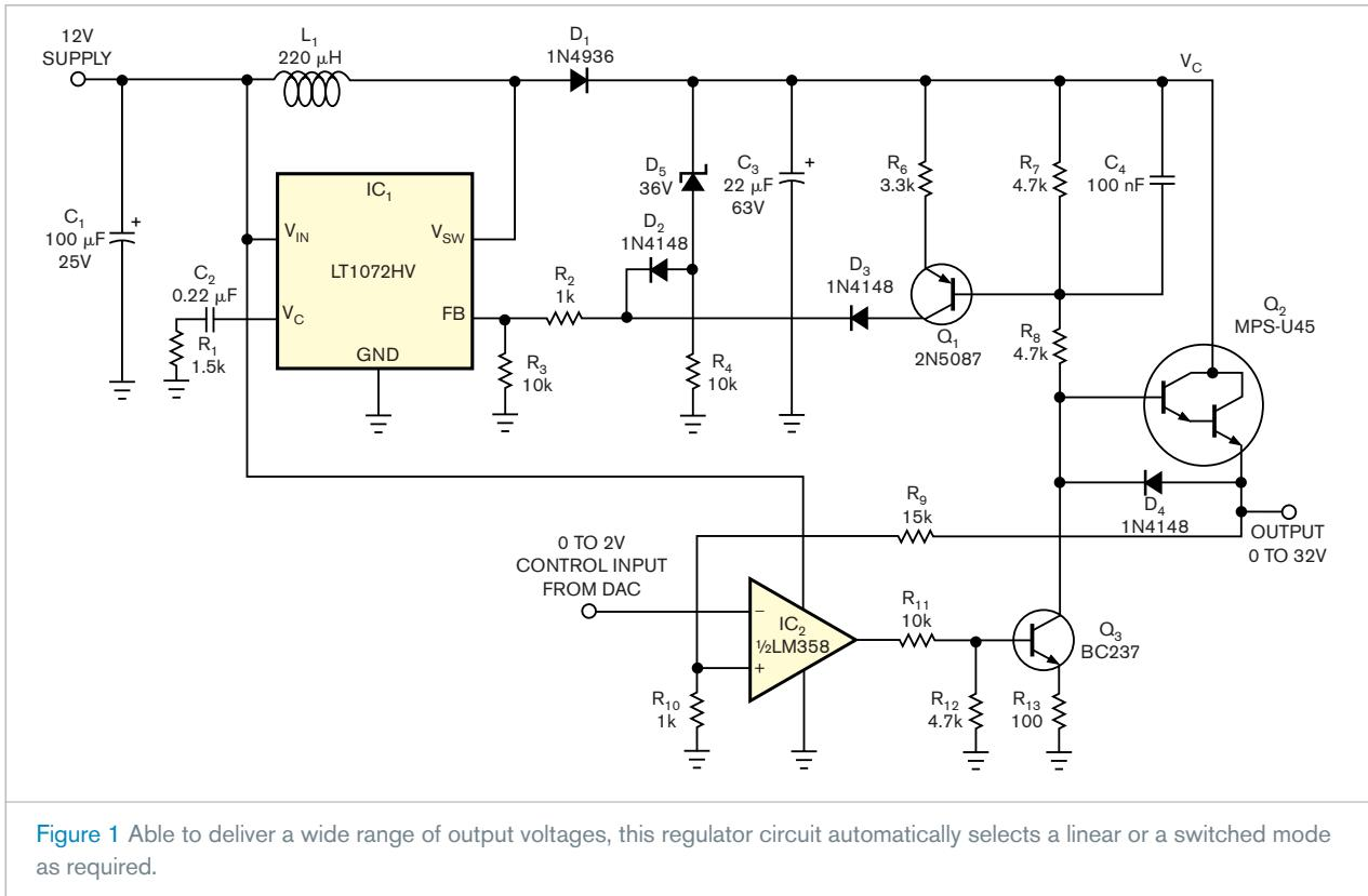
Figure 1 Able to deliver a wide range of output voltages, this regulator circuit automatically selects a linear or a switched mode as required.
