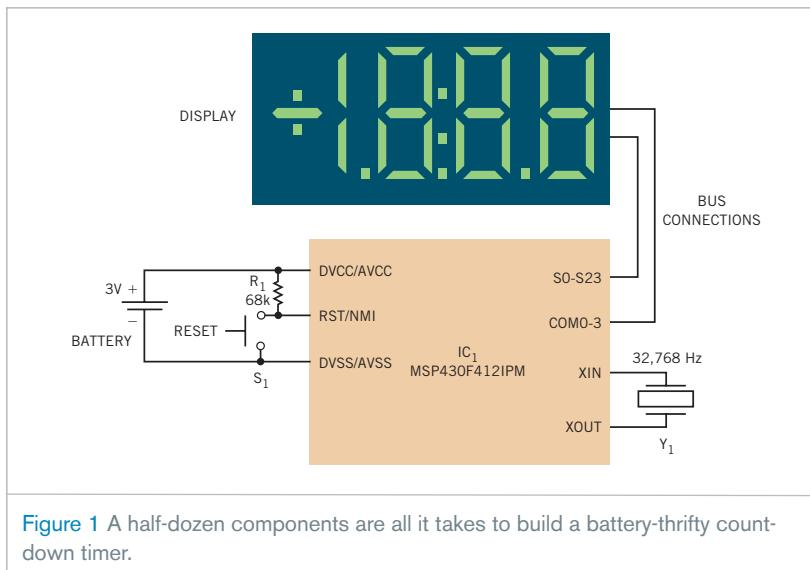
**Figure 1** A half-dozen components are all it takes to build a battery-thrifty countdown timer.
