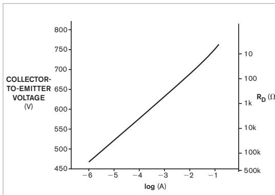
**Figure 2** A VI characteristic shows the corresponding differential-resistance graph for a short-circuited BC337-16 transistor. (Note: The -16 denotes a sorted  $h_{FE}$  range of  $100 < h_{FE} < 250$ .)
