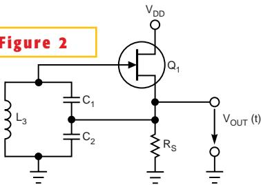
To complete the oscillator circuit, you add an LC-resonant tank to the amplifier stage; the result is a Colpitts oscillator.
