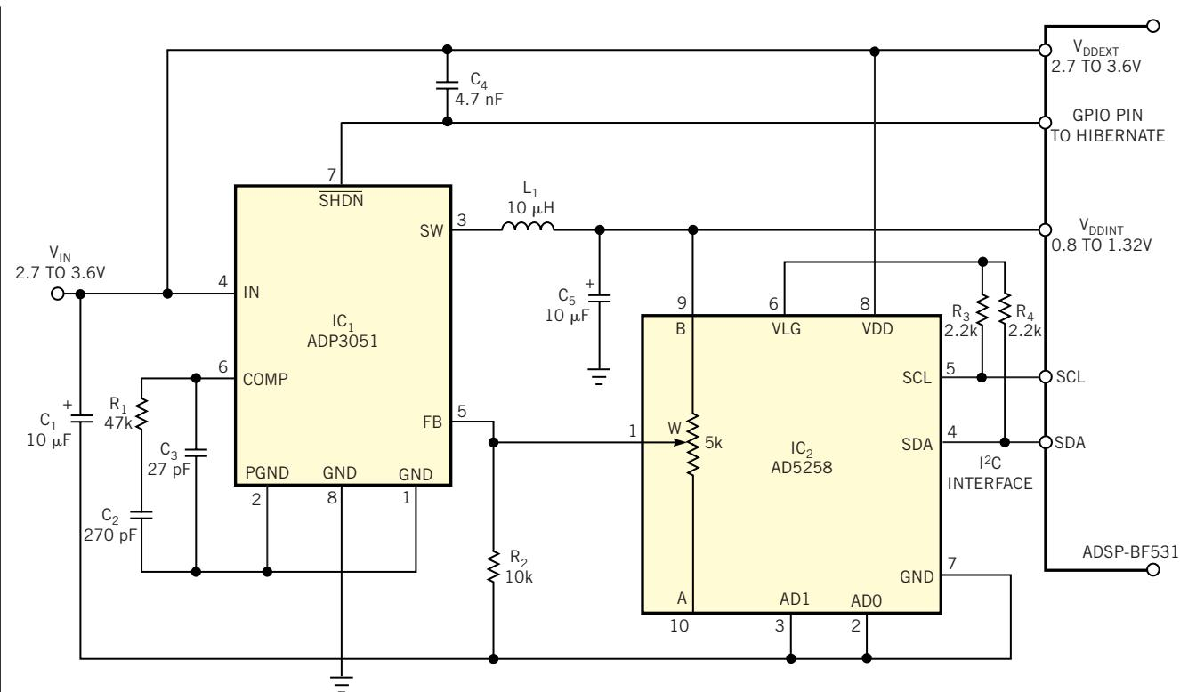
**Figure 1** Under control of its host processor, digital potentiometer IC<sub>2</sub> adjusts the processor's core power-supply voltage.
