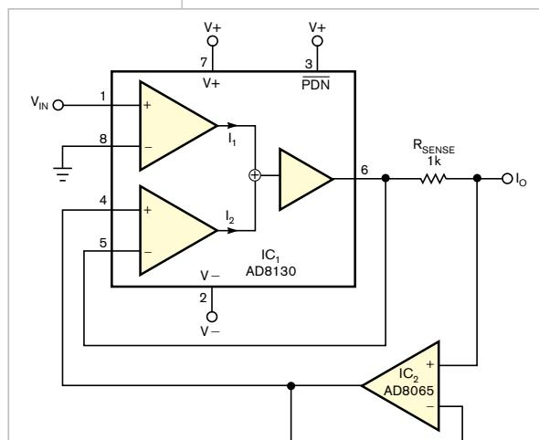
**Figure 2** Adding an Analog Devices AD8065 buffer amplifier, IC<sub>2</sub>, isolates the current-sampling resistor R<sub>SENSE</sub> and reduces errors that IC<sub>1</sub>'s input-bias current contributes.
