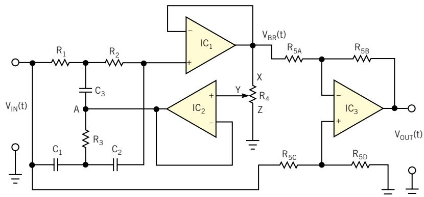
**Figure 1** This bandpass active filter features adjustable Q and maximum gain in the passband and consists of a twin-T cell with Q adjustment and a differential output stage. You can also extract a frequency-notch output from the voltage-follower stage.
