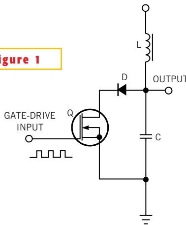
Few components are necessary to produce a pseudo sine wave.
