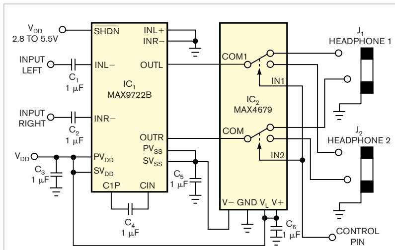
**Figure 2** Higher values of  $V_{DD}$ , 2.8 to 5.5V, require a different amplifier and a dual-supply-voltage switch at IC<sub>2</sub>.
