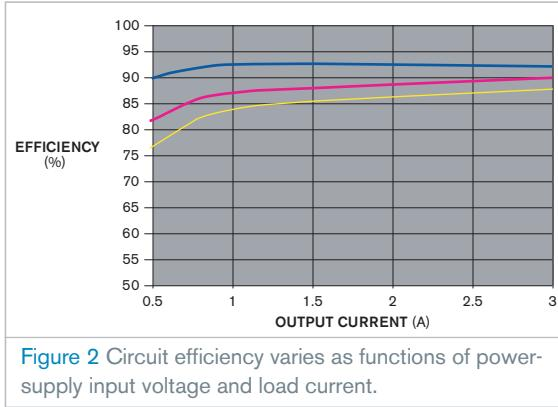
**Figure 2** Circuit efficiency varies as functions of power-supply input voltage and load current.
