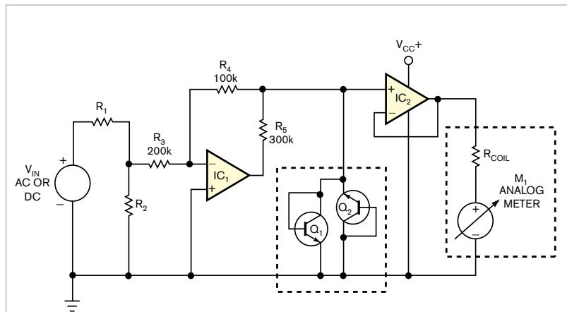
**Figure 3** Based on rail-to-rail operational amplifier  $IC_1$ , this circuit's input stage forms a diodeless, precision full-wave rectifier and enables the circuit of **Figure 2** to display ac- or dc-voltage measurements on a dc meter.
