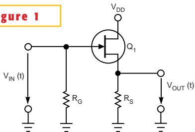
You can configure an amplifier stage, based on a JFET transistor, as a common drain.
