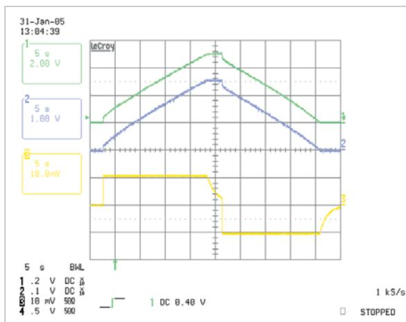
**Figure 2** The oscilloscope waveforms within the active-balance circuit show the power-supply rail voltage (top trace), the midpoint voltage at the junction between the two capacitors (middle trace), and the charge/discharge current (lower trace, scaled to 1A per division). The traces reflect a 1A charge interval to 5V, followed by a 1A discharge to 0V. The waveform steps at the start of the charge and discharge intervals are due to the capacitor's internal ESRs.
