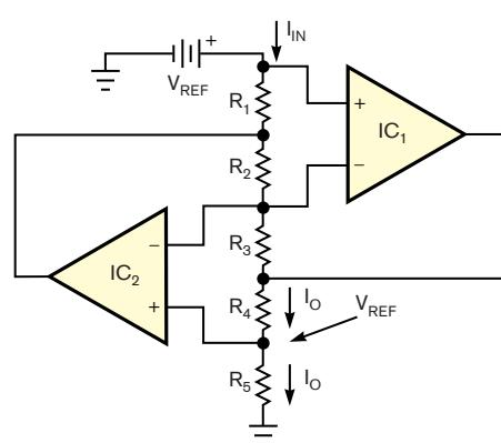
Figure 2 Replacing all of a GIC's impedances with resistors creates a constant-current source.
