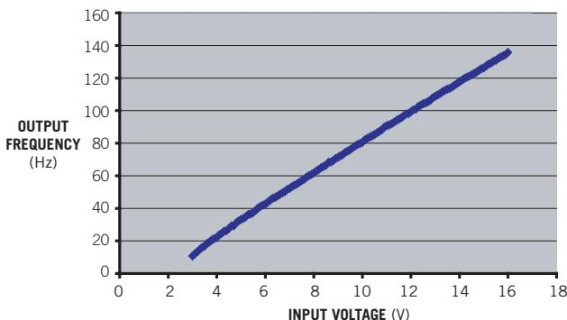
**The measured transfer function of the VFC exhibits excellent linearity over a wide range of inductively coupled input voltages.**
