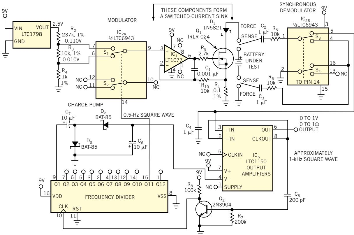
**Figure 2** This circuit determines a battery's internal resistance by repetitively applying a calibrated discharge current and measuring the resultant voltage drop across the battery's terminals.
