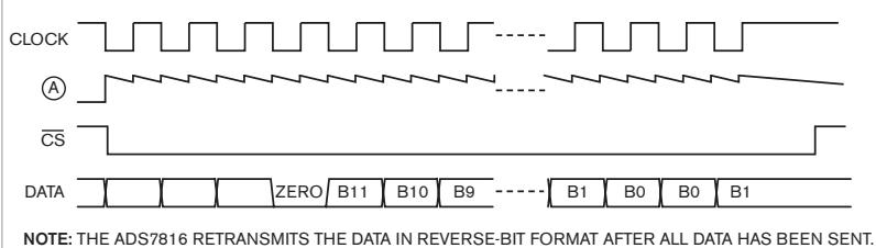
**Figure 2** An SPI-clock waveform (top trace) evokes data (bottom trace), and peak detection of the clock (the waveform at Point A in Figure 1) yields a signal (next-to-bottom trace) that mimics the chip-selection line's behavior.
