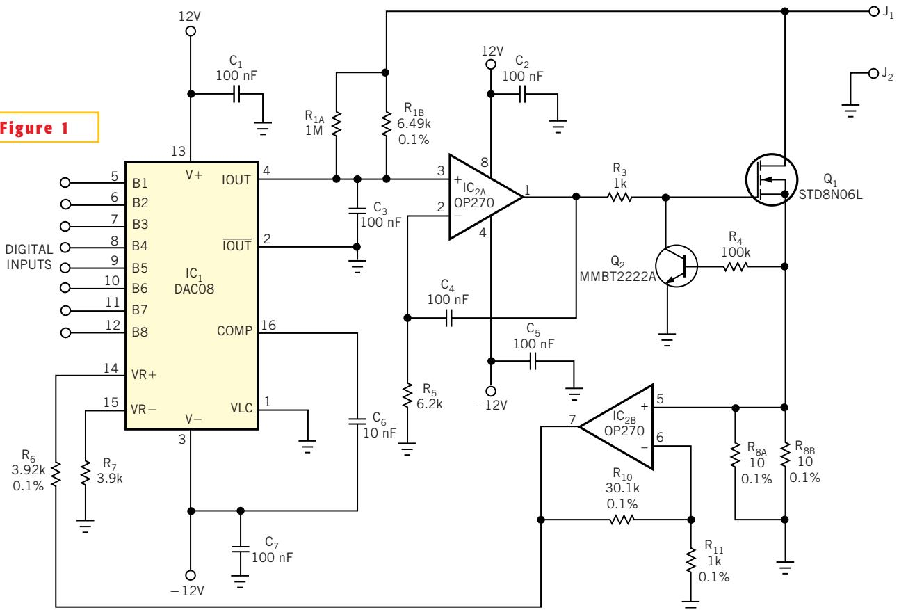
This digitally programmable resistor features low component count and inexpensive parts.
