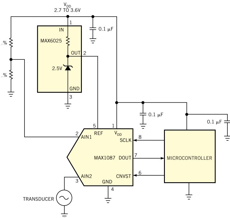
**Figure 1** To eliminate the resistive divider, you connect the ADC's reference voltage to its power supply and measure the precision voltage reference's output.
