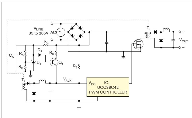
**Figure 3** In this improved design, pulse-width-controller  $IC_1$  derives its power from  $R_T$  for start-up, auxiliary winding  $W_{\text{AUX}}$  for normal operation, and shunt-regulator circuit  $IC_2$  and  $Q_1$  for low-load operation.
