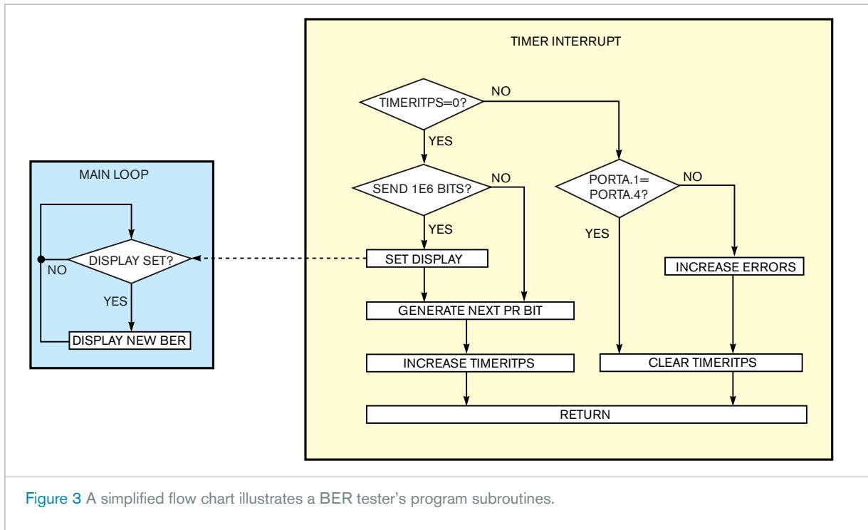
Figure 3 A simplified flow chart illustrates a BER tester's program subroutines.
