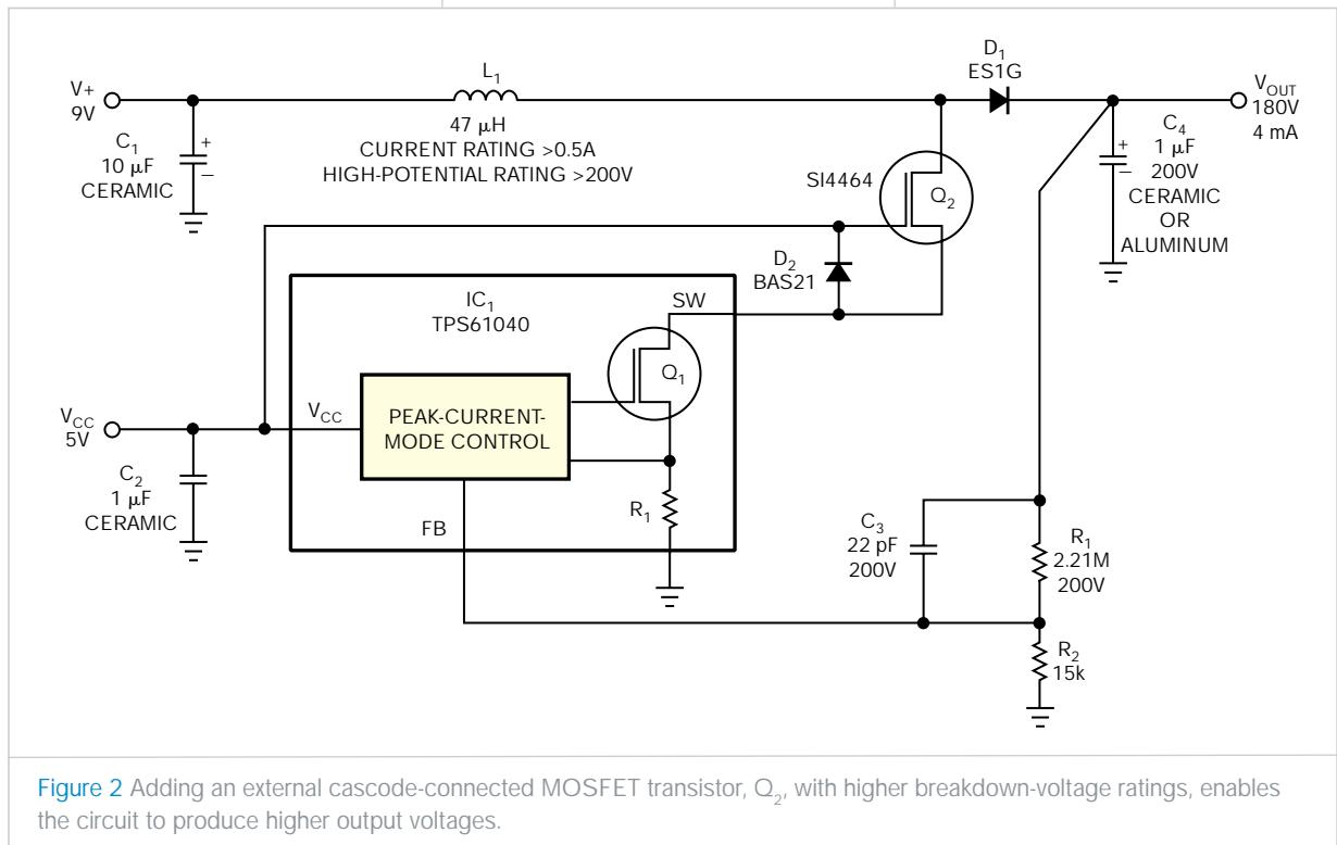
Figure 2 Adding an external cascode-connected MOSFET transistor,  $Q_2$ , with higher breakdown-voltage ratings, enables the circuit to produce higher output voltages.
