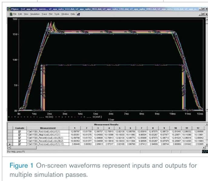
Figure 1 On-screen waveforms represent inputs and outputs for multiple simulation passes.
