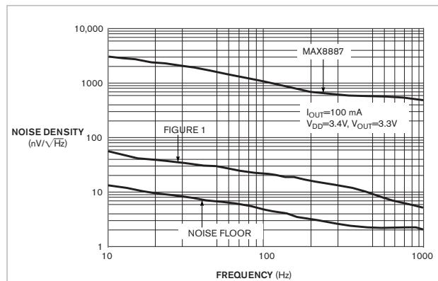
**Figure 3** A noise-density-versus-frequency plot for the low-dropout circuit in **Figure 1** is 38 dB lower than that of a conventional low-noise, low-dropout-voltage regulator—in this case, a Maxim MAX8887.
