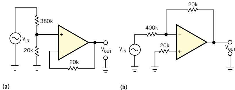
**Figure 1** To measure high voltages, you can use discrete resistors to assemble an input voltage divider and buffer (a) or an attenuating inverter (b), but performance suffers due to thermal mismatch.
