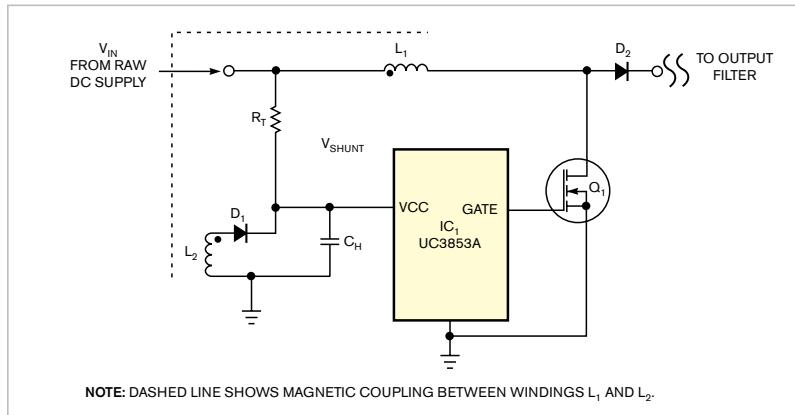
**Figure 1** In a conventional switched-mode power supply's bootstrap circuit, trickle-charge resistor R<sub>T</sub> and capacitor C<sub>H</sub> supply start-up power to the pulse-width modulator and controller, IC<sub>1</sub>.
