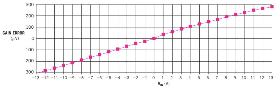
The circuit in Figure 2 introduces a full-scale gain error of less than 300  $\mu\text{V}$  over a 26V input-voltage range.
