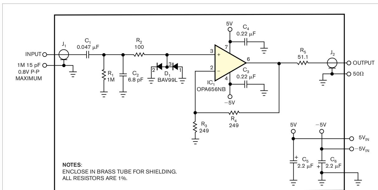
**Figure 1** Just a handful of parts can help extend a spectrum analyzer's performance. This unity-gain probe emulates a standard oscilloscope probe's  $1\text{-M}\Omega$  and  $15\text{-pF}$  input characteristics and easily drives  $50\Omega$  loads.
