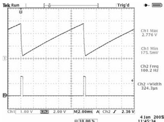
**Figure 2** Oscilloscope measurements of the VFC show voltage across capacitor  $C_5$  (upper trace) and comparator  $IC_2$ 's output voltage,  $V_{OUT}$  (lower trace), for a nominal input voltage of 12V.
