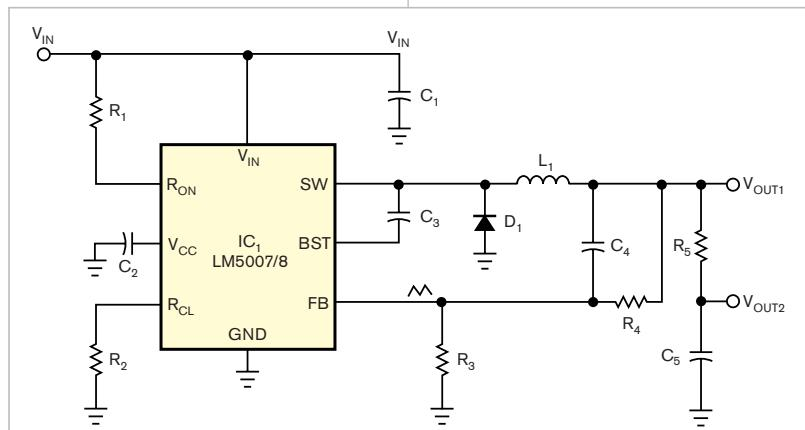
**Figure 1** This basic switched-mode voltage regulator reduces its input voltage to a lower value.
