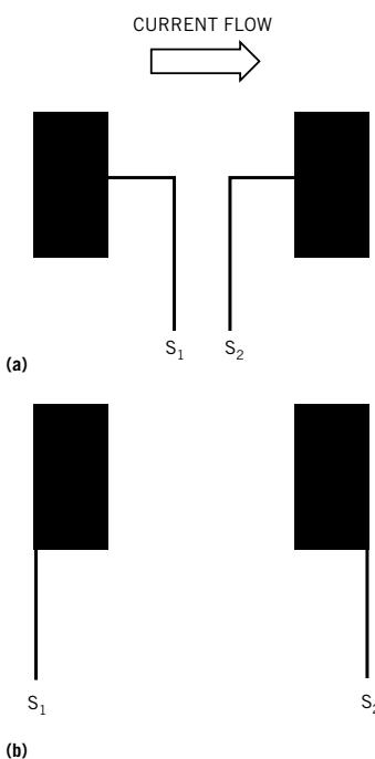
**Figure 1** Conventional solder pads offer two choices for Kelvin connections: on the pads' inner edges (a) or outer corners (b).
