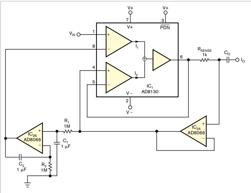
**Figure 3** For an ac-coupled current output, add a dc-stabilization loop, IC<sub>2A</sub> and IC<sub>2B</sub>.
