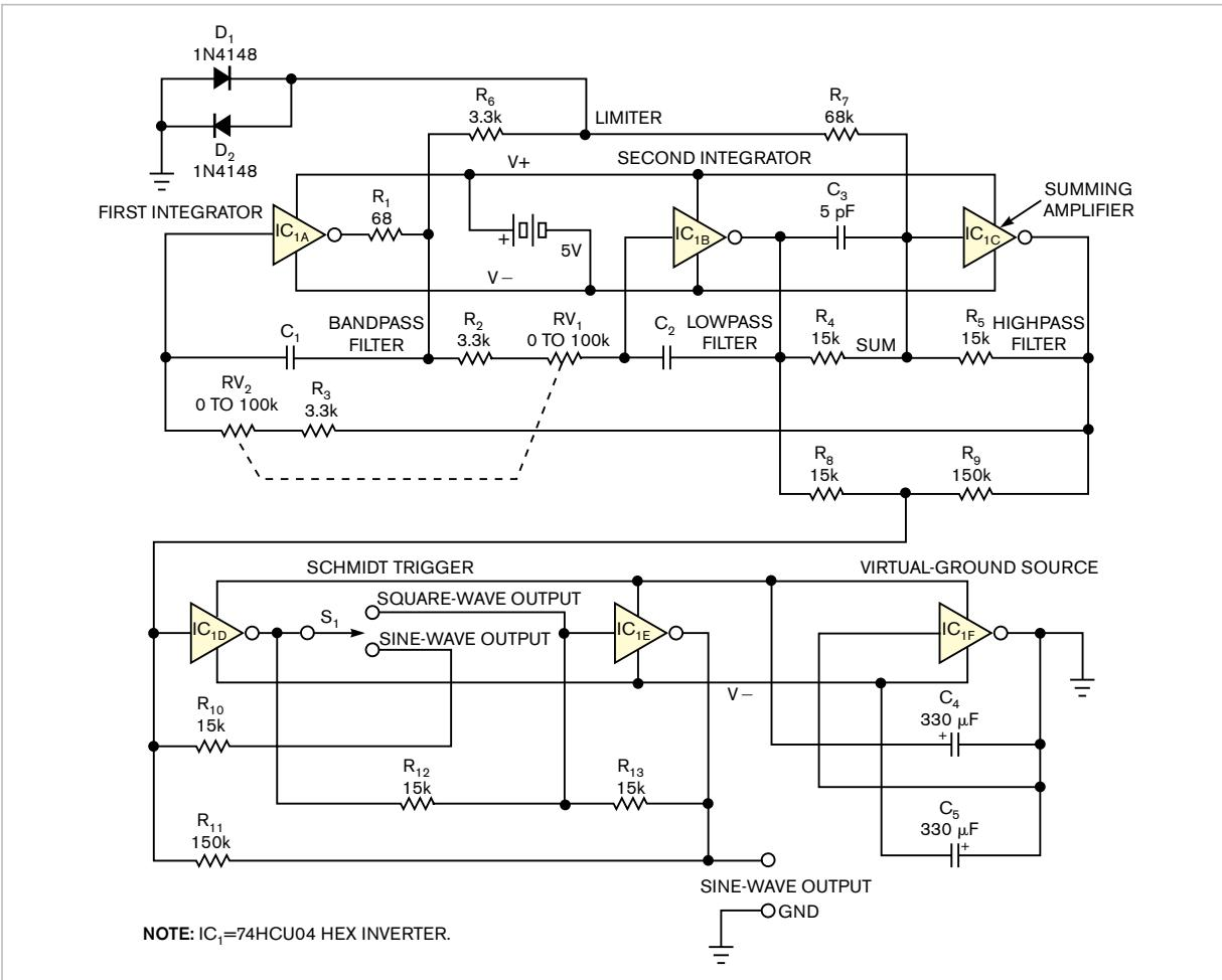
Figure 1 Build a sine-wave source around a single high-speed CMOS hex inverter and a handful of components.
