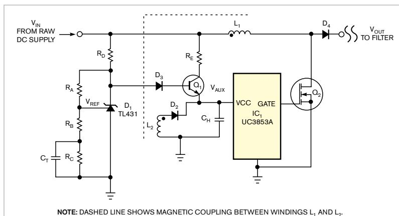
**Figure 2** In this augmented bootstrap circuit, transistor Q<sub>1</sub> delivers a robust initial pulse of current to capacitor C<sub>H</sub>, ensuring faster start-up and power delivery.
