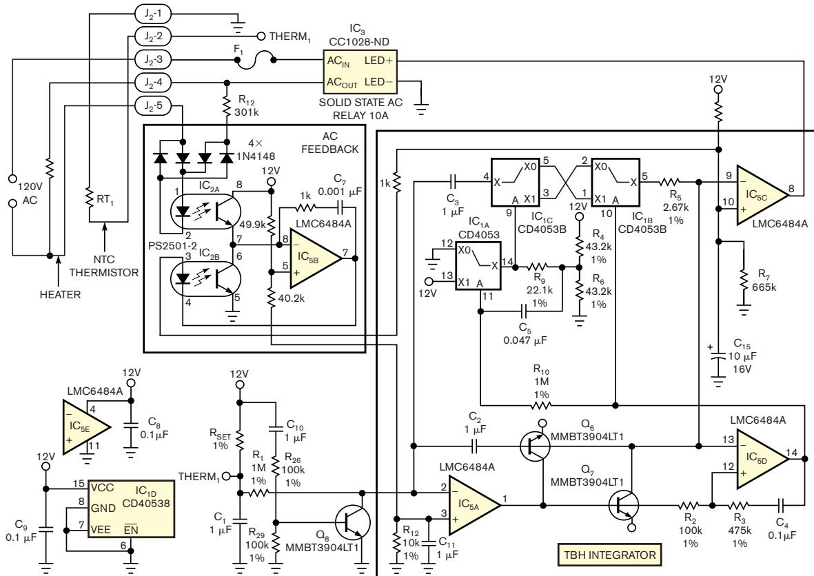
**NOTE:**  $R_5$  IS 10 TIMES THE THERMISTOR SETPOINT.
