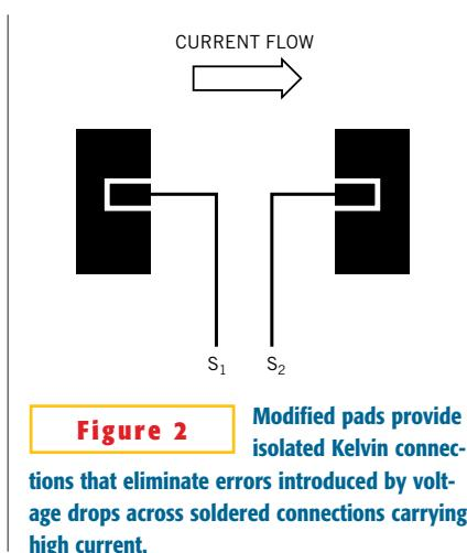
ror of 18.2%. **Figure 2** shows an improved component footprint. Each large solder pad includes a central cutout area that partially surrounds a narrow pad that solders directly to the sense element and thus carries no current. This approach removes from the sense path the large-area solder joints that mount the part and carry high load current.
