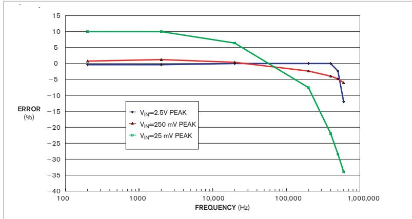
**Figure 2** Plotting the difference between peak signal levels and output voltage for three peak levels illustrates the detector's frequency response.
