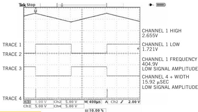
**Figure 2** This oscilloscope photo shows circuit's internal waveforms: Trace 1 is the integrator's output voltage, Trace 2 is the comparator's output voltage, Trace 3 is the inverter's output voltage, and Trace 4 is the PPM-output voltage.
