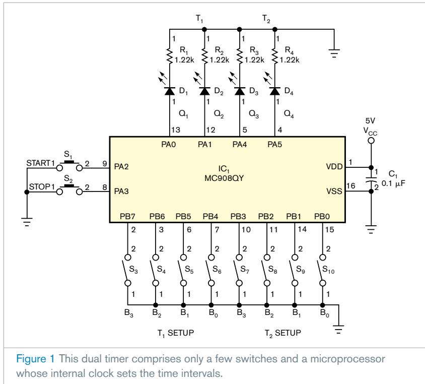
**Figure 1** This dual timer comprises only a few switches and a microprocessor whose internal clock sets the time intervals.
