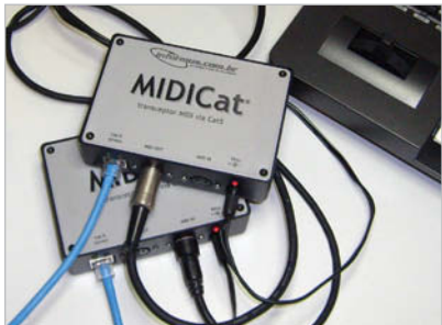
Figure 1 You can test the completed MIDI drivers with a 100m Category 5 cross cable.
