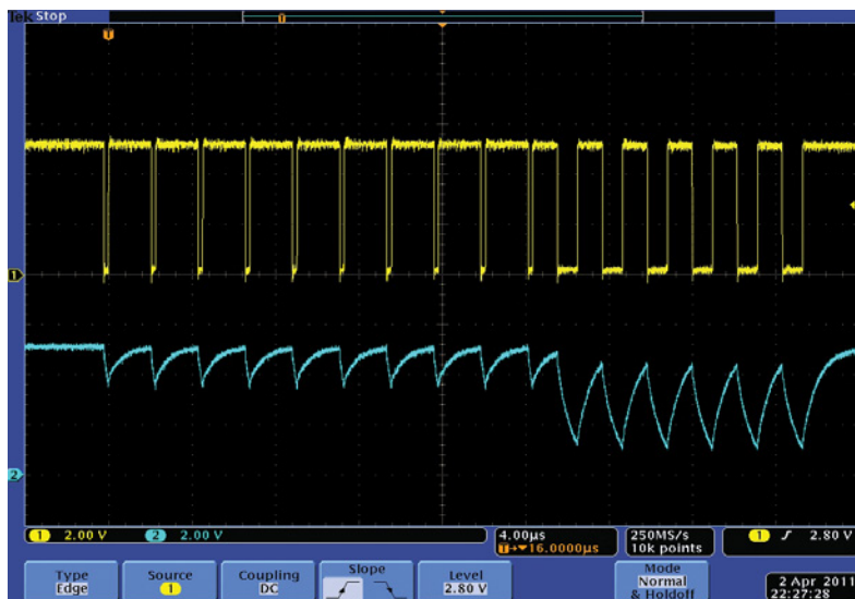
Figure 3 The waveform shows the circuit writing the pattern 1111111111000000 for the display. The upper, yellow trace is the clock signal, and the lower, blue trace is the data signal.
