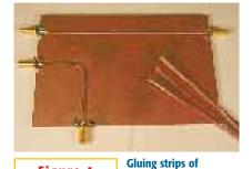
Figure 1 RT/duroid material on top of normal FR4 pc-board material makes a very quick Microstrip structure. Make sure that the line lies flat and is firmly glued in place against the board to maximize the return loss
