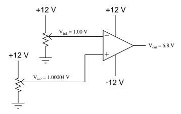
Also, write a mathematical formula solving for differential voltage gain  $(A_V)$  in terms of an op-amp's input and output voltages.
