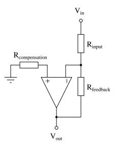
Explain what this "compensation" resistor is compensating for, and also what its value should be.  $\underline{\text{file }01007}$
