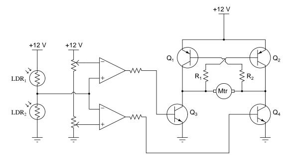
In this circuit, what guarantees that the two comparators never output a "high" (+V) voltage simultaneously, thus attempting to move the tracking motor clockwise and counter-clockwise at the same time?  $\frac{\text{file }00881}{\text{file }00881}$
