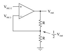
Then, once you have an equation written, solve for the output voltage if the noninverting input voltage is -2.4 volts.
