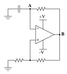
Explain how this circuit works, and what waveforms will be measured at points A and B.  $\underline{\text{file }01171}$
