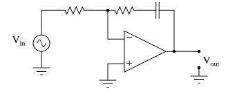
What type of filtering function (low pass, high pass, band pass, band stop) is provided by both these filter circuits? Comparing these two circuit designs, which one do you think is more practical? Explain your answer.
