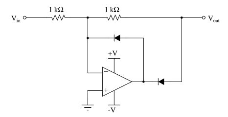
Assume that both diodes in this circuit are silicon switching diodes, with a nominal forward voltage drop of 0.7 volts.
