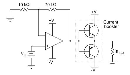
However, if connected exactly as shown, there will be a significant voltage error introduced to the opamp's output. No longer will the final output voltage (measured across the load) be an exact 3:1 multiple of the input voltage, due to the 0.7 volts dropped by the transistor in active mode:
