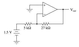
Also, calculate the DC voltage gain of this circuit. file 00932
