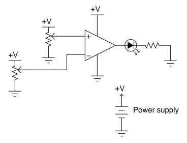
Trace the complete path of current powering the LED. Where, exactly, does the LED get its power from?
