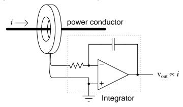
Explain why an integrator circuit is necessary to condition the Rogowski coil's output so that output voltage truly represents conductor current.
