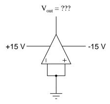
In reality, the output voltage of an op-amp under these conditions is not the same as what would be ideally predicted. Identify the fundamental problem in real op-amps, and also identify the best solution. file 00847
