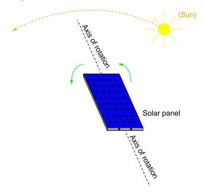
One way to detect the sun's position relative to the panel is to attach a pair of Light-Dependent Resistors (LDR's) to the solar panel in such a way that each resistor will receive an equal amount of light only if the panel is pointed directly at the sun:
