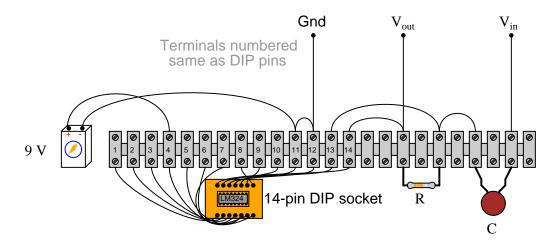
Challenge question: given the single-supply configuration (+9 volts only), this differentiator circuit can only respond to one direction of input voltage change  $(\frac{dv_{in}}{dt})$ . Which direction is this: positive or negative?
