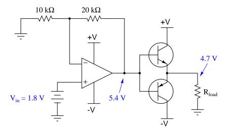
There is a very simple way to completely eliminate this error, without adding any additional components. Modify the circuit accordingly.
