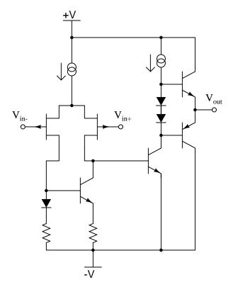
Qualitatively determine what will happen to the output voltage  $(V_{out})$  if the voltage on the noninverting input  $(V_{in+})$  increases, and the voltage on the inverting input  $(V_{in-})$  remains the same (all voltages are positive quantities, referenced to -V). Explain what happens at every stage of the op-amp circuit (voltages increasing or decreasing, currents increasing or decreasing) with this change in input voltage.
