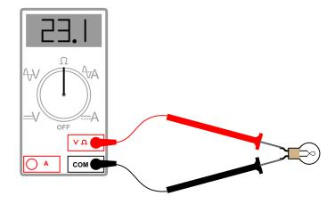
Also, identify the reading you would expect the ohmmeter to indicate if the light bulb were burnt out (failed "open"). <u>file 00101</u>
