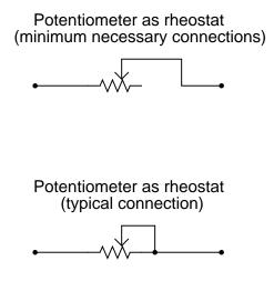
Explain what advantage is gained by connecting the wiper to the unused terminal. Why is the lower potentiometer connection scheme more commonly used than the upper?
