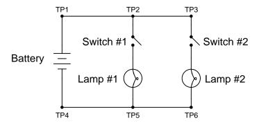
Identify which of these hypothetical faults could account for this problem, and which could not account for the problem. In other words, which of these faults are possible, and which are not possible, given the symptoms exhibited by the circuit? Consider each of these hypothetical faults one at a time (no multiple, simultaneous faults):
