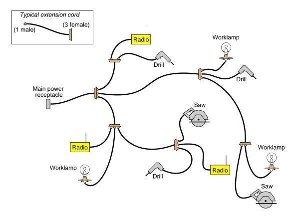
Despite this dangerous wiring, all tools have functioned so far without trouble. Then suddenly both the worklight and the circular saw in the lower-right corner of the illustration stop working. All the other tools continue to function properly (including all the radios, which is very fortunate because the workers become irritable without their music).
