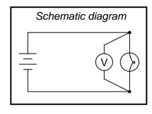
In order to practically function, an voltmeter must have some finite amount of internal resistance. It is usually a very large amount, but less than infinite. It should be apparent to you that the presence of this resistance will have some effect on the circuit voltage, when compared to the amount of voltage in the circuit without any meter connected, due to the fact that real voltage sources tend to "sag" when subjected to additional loads:
