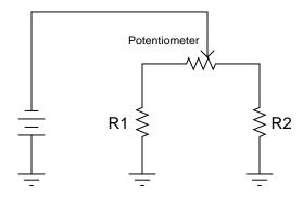
Which way would you have to twist the potentiometer shaft in order to increase current through resistor R1, clockwise or counter-clockwise? Explain your answer.
