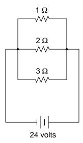
Explain, step by step, how to calculate the amount of current (I) that will go through each resistor in this parallel circuit, and also the voltage (V) dropped by each resistor:
