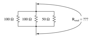
No, this is not a "trick" question! There is a way to apply a two-resistance equation to solve for three resistances connected in parallel.
