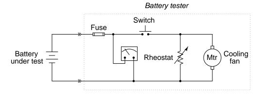
Other clues to the problem include the fact that rheostat setting seems to make no difference in the voltmeter's indication, and also that the cooling fan motor does not come on when the switch is pressed.
