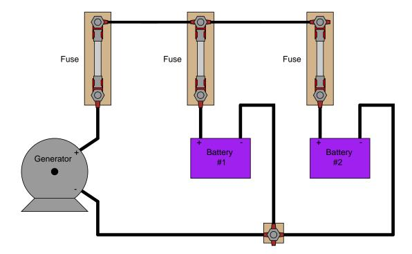
To do so, of course, you need to determine the direction of current through each battery. Unfortunately, your multimeter does not have the current rating necessary to directly measure such large currents, and you do not have access to a clamp-on (magnetic) ammeter capable of measuring DC current.
