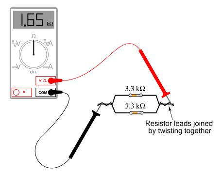
Follow-up question: how much resistance would you expect the ohmmeter to register if there were *three* similarly-sized resistors connected in parallel instead of two? What if there were *four* resistors?
