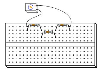
The interconnections between the metal spring clips within the holes of the breadboard allow continuity between adjacent leads of the resistors, without the resistor leads having to be jammed into the same hole.
