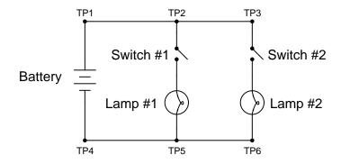
Identify which of these hypothetical faults could account for this problem, and which could not account for the problem. In other words, which of these faults are possible, and which are not possible, given the symptoms exhibited by the circuit? Consider each of these hypothetical faults one at a time (no multiple, simultaneous faults):
