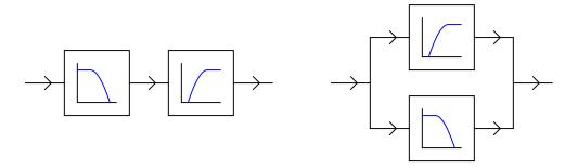
Plot the typical response of a band-pass filter circuit, showing signal output (amplitude) on the vertical axis and frequency on the horizontal axis:
