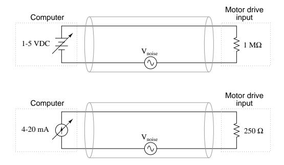
Use the superposition theorem to qualitatively determine which signal standard drops the greatest amount of noise voltage across the motor drive input's resistance, thereby most affecting the motor speed control.
