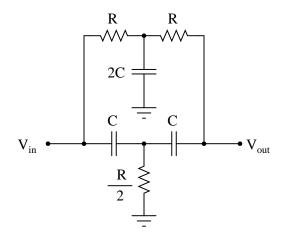
Research the equation predicting this circuit's "notch" frequency, given the component value ratios shown.
