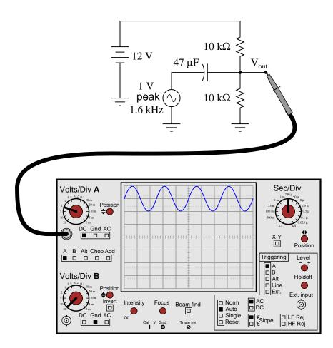
Follow-up question: what would the oscilloscope display look like if the coupling switch for channel A had been set to "AC" instead of "DC"?
