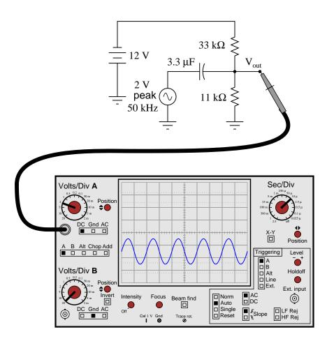
Follow-up question: explain why it is acceptable to use a polarized (polarity-sensitive) capacitor in this circuit when it is clearly connected to a source of AC. Why is it not damaged by the AC voltage when used like this?
