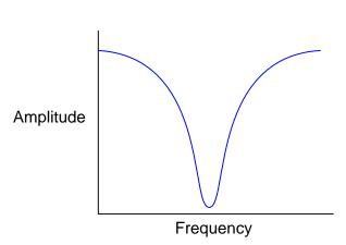
The bandwidth of a band-stop filter circuit is that range of frequencies where the output amplitude is reduced to at least 70.7% of full attenuation:
