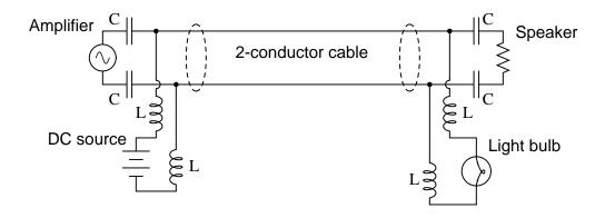
Apply the Superposition Theorem to this circuit to demonstrate that the audio and DC signals will not interfere with each other as they would if directly connected. Assume that the capacitors are of such large value that they present negligible impedance to the audio signal  $(Z_C \approx 0 \Omega)$  and that the inductors are sufficiently large that they present infinite impedance to the audio signal  $(Z_L \approx \infty)$ . <u>file 01856</u>
