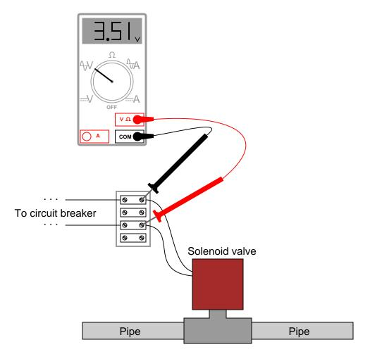
Now, three and a half volts AC is not enough voltage to cause any harm, but its presence confuses and worries the technician. Shouldn't there be 0 volts, with the breaker turned off?
