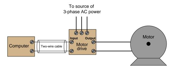
Two common standards for analog control signals are 1-5 volts DC and 4-20 mA DC. In either case, the motor will spin faster when this signal from the computer grows in magnitude (1 volt = motor stopped, 5 volts = motor runs at full speed; or 4 mA = motor stopped, 20 mA = motor runs at full speed).
