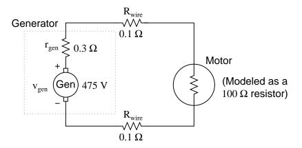
Calculate the amount of current this generator will supply to the motor and the voltage measured across the motor's terminals, taking into account all the resistances shown (generator internal resistance  $r_{gen}$ , wiring resistances  $R_{wire}$ , and the motor's equivalent resistance).
