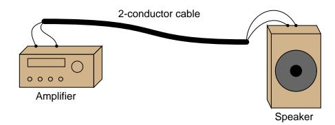
This system may be schematically modeled as an AC voltage source connected to a load resistor:
