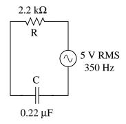
Show mathematically how the resistance and reactance combine in series to produce a total impedance (scalar quantities, all). Then, show how to analyze this same circuit using complex numbers: regarding each of the component as having its own impedance, demonstrating mathematically how these impedances add up to comprise the total impedance (in both polar and rectangular forms).
