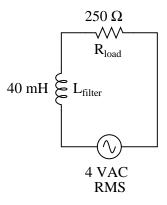
What do these figures tell you about the nature of this filter circuit (whether it is a low-pass or a high-pass filter), and also about the definition of *cutoff frequency* (also referred to as  $f_{-3dB}$ )? <u>file 00646</u>
