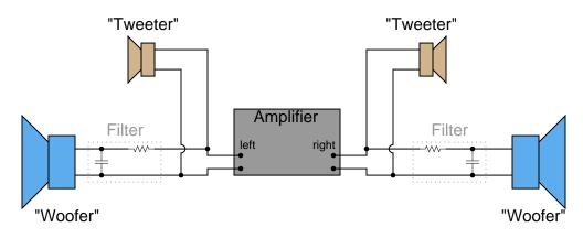
After examining this schematic, you see that your friend has the right idea in mind, but implemented it incorrectly. These filter circuits would indeed block high-frequency signals from getting to the woofers, but they would not actually accomplish the stated goal of minimizing wasted power.
