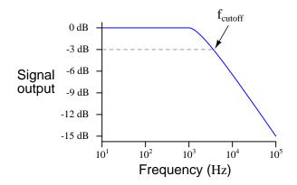
What does the term *rolloff* refer to, in the context of filter circuits and Bode plots? Why would this parameter be important to a technician or engineer? <u>file 01246</u>
