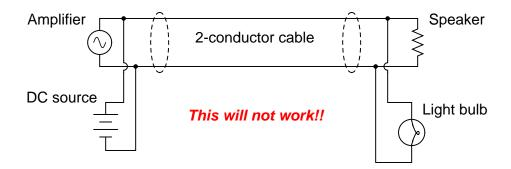
If we were to connect the components together as shown above, the DC power source will likely damage the amplifier by being directly connected to it, the speaker will *definitely* be damaged by the application of significant DC voltage to its coil, and the light bulb will waste audio power by acting as a second (non-audible) load. Suffice to say, this is a bad idea.
