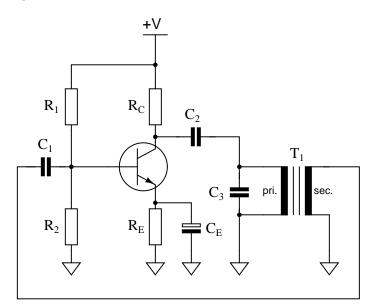
How would this effective decreasing of the primary winding turns affect the operation of this circuit? What if it were the secondary winding of the transformer to suffer this fault instead of the primary?  $\frac{\text{file } 03757}{\text{file } 03757}$
