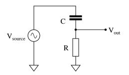
He recognizes this as a series circuit, and therefore realizes that a right triangle would be appropriate for representing component impedances and component voltage drops (because both impedance and voltage are quantities that add in series, and the triangle represents phasor addition):
