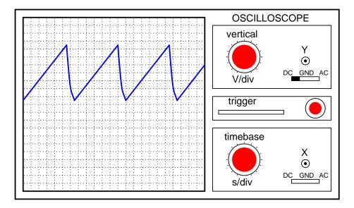
What function does the JFET perform in this circuit, based on your analysis of the new TP1 signal waveform? The straight-line charging voltage pattern shown on the second oscilloscope display indicates what the JFET is doing in this circuit.
