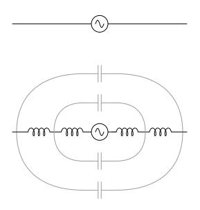
Follow-up question: how would you expect the inductance and capacitance of this antenna to relate to its physical length? In other words, as you increase the length of an antenna, would its inductance increase or decrease? As the length increases, would its capacitance increase or decrease? Explain your reasoning.
