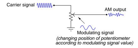
Now, such a potentiometer circuit would be totally impractical for any modulating signal frequency measured in Hertz, as the potentiometer would wear out very rapidly from all the motion. It is the *principle* of modulated voltage division that this circuit helps to communicate, though. Multiplier circuits do the same thing, only multiplying the amplitude of the carrier signal rather than dividing it.
