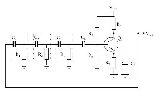
What must the voltage gain be for the common-emitter amplifier if the total voltage attenuation for the three phase-shifting RC networks is -29.25 dB?
