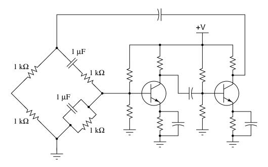
Explain why the operating frequency will not be the same if the transistor receives its feedback signal from the other side of the bridge, like this:
