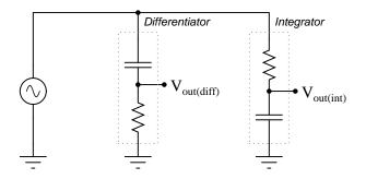
If, however, the excitation voltage is slightly distorted, one of the outputs will be more sinusoidal than the other. Explain whether it is the differentiator or the integrator that produces the signal most resembling a pure sine wave, and why.
