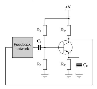
We know that oscillator circuits require "regenerative" feedback in order to continuously sustain oscillation. Explain how the correct amount of phase shift is *always* provided in the feedback circuit to ensure that the nature of the feedback is always regenerative, not degenerative. In other words, explain why it is not possible to incorrectly choose feedback network component values and thus fail to achieve the proper amount of phase shift.
