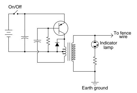
A technician does some troubleshooting and determines that the transistor is defective. She replaces the transistor, and the circuit begins to work again, its rhythmic output pulses indicated by the neon lamp.
