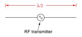
Also, calculate the practical antenna length considering the "end effect," which makes the antenna's electrical length slightly different from its physical length (assume a K factor of 0.95). <u>file 02281</u>
