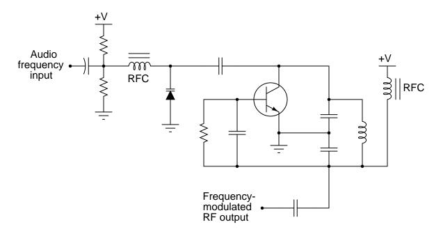
The oscillator is of the "Colpitts" design. The key to understanding this circuit's operation is knowing how the *varactor* diode responds to different amounts of DC bias voltage. Explain how this circuit works, especially how the diode exerts control over the oscillation frequency. Why does the output frequency vary as the control voltage varies? Does the output frequency increase or decrease as the control voltage input receives a more positive voltage?
