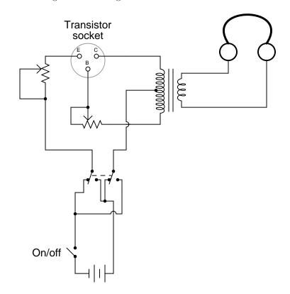
After repairing a broken solder joint, the technician notices that the DPDT switch has lost its label. The purpose of this switch is to allow polarity to be reversed so as to test both PNP and NPN transistor types. However, the label showing which direction is for NPN and which direction is for PNP has fallen off. And, to make matters worse, the schematic diagram does not indicate which position is which.
