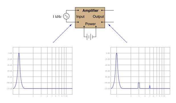
Interpret the two graphical displays and explain why the output signal has more "peaks" than the input. What is this difference telling us about the amplifier's performance?  $\frac{file\ 03307}{file\ 03307}$
