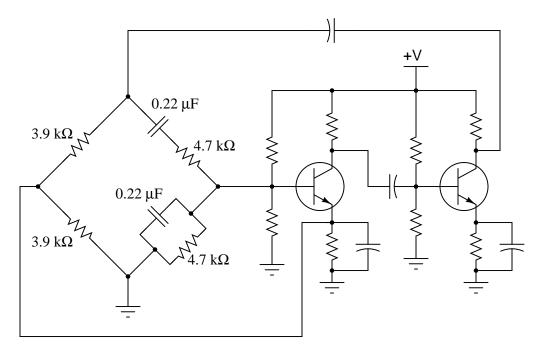
If one side of the Wien bridge is made from a potentiometer instead of two fixed-value resistors, this adjustment will affect both the *amplitude* and the *distortion* of the oscillator's output signal:
