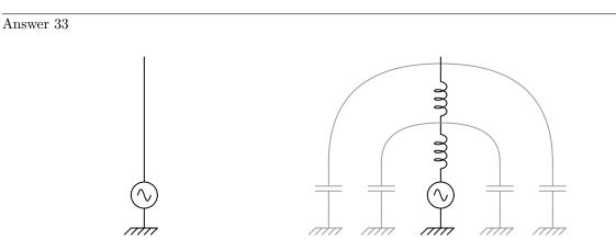
Follow-up question: how would you expect the inductance and capacitance of this antenna to relate to its physical length? In other words, as you increase the length of an antenna, would its inductance increase or decrease? As the length increases, would its capacitance increase or decrease? Explain your reasoning.
