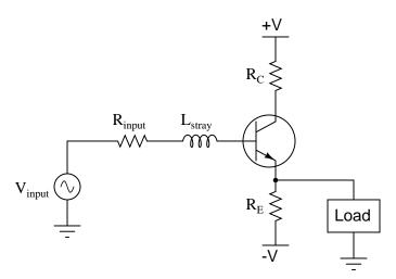
Explain how this is possible. What parasitic effects could possibly turn an amplifier into an oscillator? file 01085
