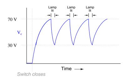
Follow-up question: assuming a source voltage of 100 volts, a resistor value of 27 k $\Omega$ , and a capacitor value of 22  $\mu$ F, calculate the amount of time it takes for the capacitor to charge from 30 volts to 70 volts (assuming the neon bulb draws negligible current during the charging phase).
