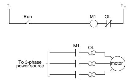
Although the "heater" elements are connected in series with the motor lines as fuses would be, they are *not* fuses! In other words, it is not the purpose of an overload heater to burn open under an overcurrent fault condition, although it is possible for them to do so.
