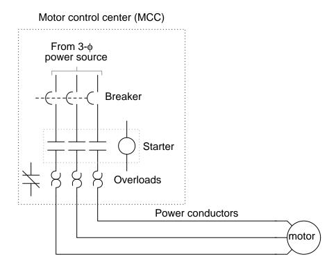
Since it is impossible for a technician to be in two places at once, it is often necessary to perform diagnostic checks on a malfunctioning electric motor from the MCC where the technician has access to all the control circuitry.
