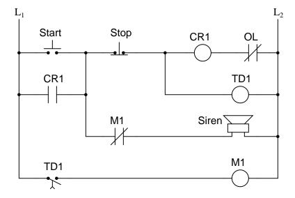
However, this circuit is poorly designed. Although it works just fine under normal conditions, it may not do what it should in the event of an overload heater trip (if the normally-closed "OL" contact opens). Explain what is wrong with this circuit.
