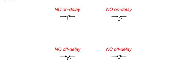
Follow-up question: how do you make sense of the arrow in each contact symbol, with regard to whether the contact is an "on-delay" or an "off-delay"?
