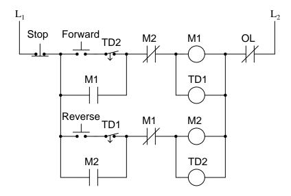
What extra functionality do the time-delay relays contribute to this motor control circuit?  $\underline{\text{file }03148}$
