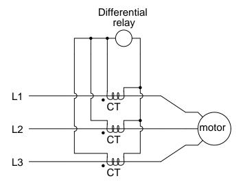
Also, explain what this relay will do to protect the circuit if it detects this kind of fault.  $\underline{\text{file }04024}$
