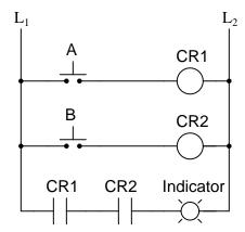
How do we know which relay contact is actuated by which relay coil? How does this convention differ from that of standard electrical/electronic schematic diagrams, where the relay coil is shown as an actual coil of wire (inductor symbol) with the contact "linked" to the coil by a dashed line? Also, what type of logic function behavior (AND, OR, NAND, or NOR) does the above circuit exhibit?
