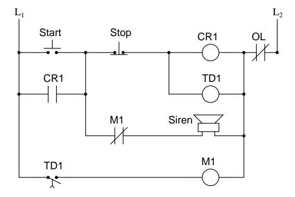
Unfortunately, there is a problem somewhere in this circuit. Instead of activating the siren before starting the motor, there is silence. The motor's start is still delayed by the correct amount of time, but the siren never makes a sound. Identify some possible causes of this problem. Also, identify portions of the circuit you know to be functioning properly.
