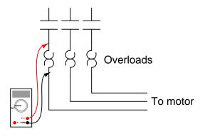
Across each overload heater element he measures about 20 mV AC with the starter engaged. From this he determines that the motor is *not* single-phasing, but is drawing approximately equal current on all three phases.
