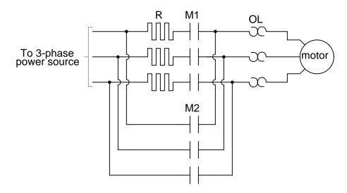
Analyze this ladder logic diagram, and explain how it starts up the electric motor more gently than an "across-the-line" starter would.
