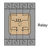
(Dashed lines represent connections between relay terminals and socket screw lugs, hidden from sight)
