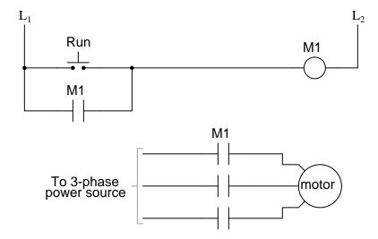
Also, explain the operation of this motor control circuit. What happens when someone actuates the "Run" switch? What happens when they let go of the "Run" switch? file 00835
