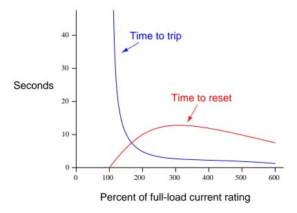
Why is there any time required to re-set an overload heater contact after a "trip"? Circuit breakers can be re-closed mere moments after a trip with no problem, and fuses (of course) can be replaced moments after blowing. Is this an intentional design feature of overload heaters, or just an idiosyncrasy?
