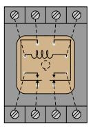
(Dashed lines represent connections between relay terminals and socket screw lugs, hidden from sight)
