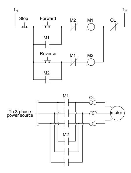
Study this diagram, then explain how motor reversal is accomplished. Also, identify the function of each "M" contact in the control circuit, especially those normally-closed contacts in series with the motor starter coils.
