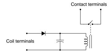
Explain how this circuit works, and also determine what type of time-delay relay function is provided by it (NOTO, NOTC, NCTO, or NCTC).
