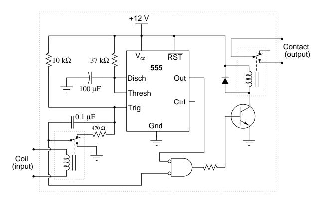
Also, calculate the amount of delay, in seconds. Hint: the 555's timing capacitor will charge from 0 volts to  $\frac{2}{3}$  supply voltage during the charging cycle.
