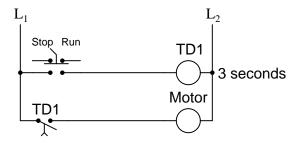
In this circuit, the motor delays start-up until three seconds *after* the switch is thrown to the "Run" position, but will stop immediately when the switch is returned to the "Stop" position. The relay contact is referred to as *normally-open*, *timed-closed*, or NOTC. It is alternatively referred to as a *normally-open*, on-delay contact.
