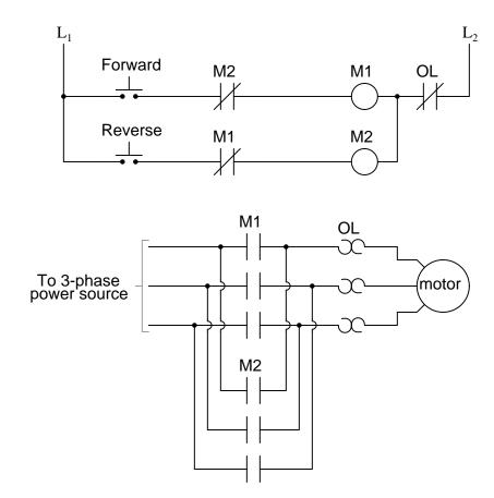
Explain how the reversal of motor direction is accomplished with two different motor starters, M1 and M2. Also, explain why there is only one set of overload heaters instead of two (one for forward and one for reverse). Finally, explain the purpose of the normally-closed contacts in series with each starter coil.
