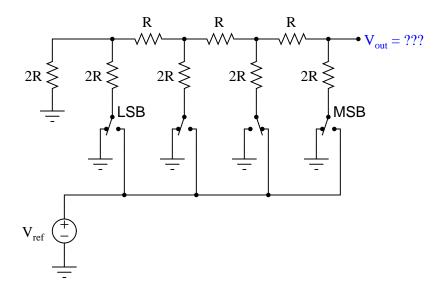
If we Thévenize all sections to the left of the activated section, replacing it with a single resistance to ground, we see the network becomes far simpler:
