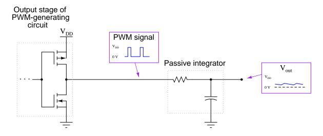
Determine the relationship between the PWM signal's duty cycle and the DC voltage output by the integrator. What does this suggest about PWM as a means of communicating information, such as analog data from a measuring device?
