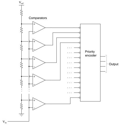
Explain why we must use a *priority* encoder to encode the comparator outputs into a four-bit binary code, and not a regular encoder. What problem(s) would we have if we were to use a non-priority encoder in this ADC circuit?
