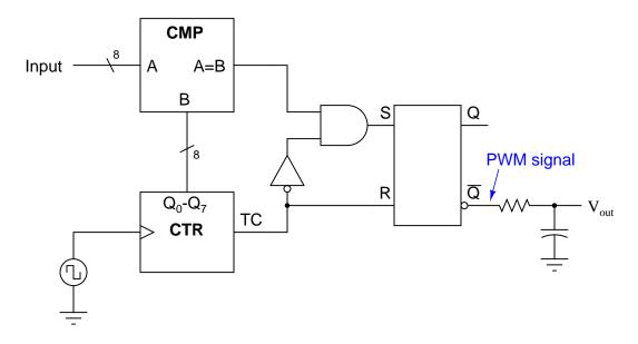
Explain how this circuit works, using timing diagrams if necessary to help show the PWM signal at  $\overline{Q}$  for different input values.
