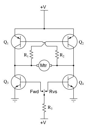
At any given moment, how many transistors are turned on and how many are turned off? Also, explain what would happen to the function of the circuit if resistor R1 failed open.  $\frac{\text{file }00449}{\text{file }00449}$
