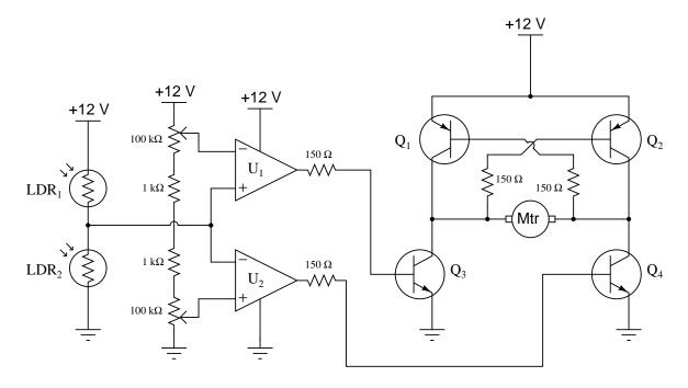
In this circuit, what guarantees that the two comparators never output a "high" (+V) voltage simultaneously, thus attempting to move the tracking motor clockwise and counter-clockwise at the same time?
