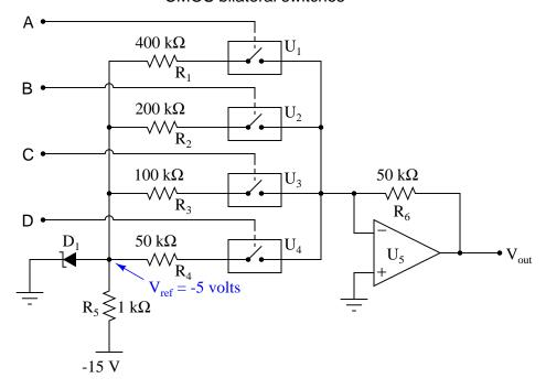
A type of resistor network known as an R-2R ladder is often used in digital-to-analog conversion circuits:
