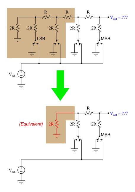
Explain how we may apply Thévenin's theorem once again to the shaded section of this next circuit (simplified from the previous circuit shown above) to simplify it even more, obtaining a final result for  $V_{out}$ :
