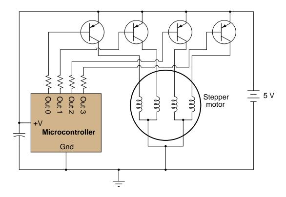
Each motor coil draws a relatively heavy current when energized, necessitating transistors to "interpose" between the microcontroller outputs and the motor coils.
