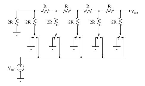
When all switches in the R-2R ladder are in the "ground" position, the network has a very interesting property regardless of its size. Analyze the Thévenin equivalent resistance (as seen from the output terminal) of the following R-2R ladder networks, then comment on the results you obtain:
