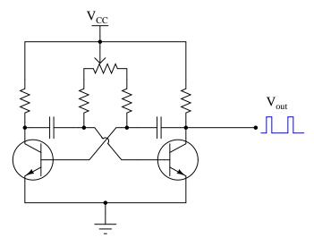
A student desires to use this circuit as the basis for a *pulse-width modulation* (PWM) power controller, to vary the amount of power delivered to a DC load. Since the oscillator circuit is built to produce weak signals and not deliver power directly to a load, the student adds a power MOSFET to switch heavy load currents:
