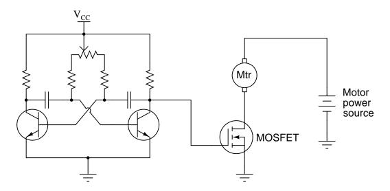
Correlate the duty cycle of the oscillator's output signal with motor power. In other words, describe how increases and decreases in signal duty cycle affect the amount of power delivered to the electric motor.  $\underline{\text{file }02152}$
