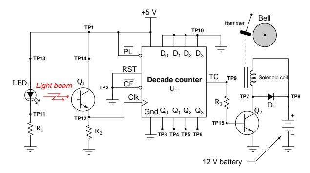
You begin troubleshooting by taking voltage measurements while people randomly enter the room (breaking the light beam as they do). Using your voltmeter, you measure a constant +5 volts at TP3 with respect to ground. This voltage measurement does not change, no matter how many people pass through the light beam. You then connect your voltmeter between TP12 and ground, measuring approximately 0 volts all the time whether or not someone is passing through the doorway.
