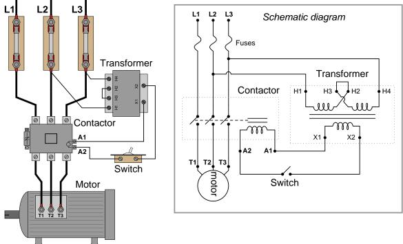
Using your AC voltmeter, you measure 476 volts AC between L1 and L2, 477 volts AC between L2 and L3, and 475 volts AC between L1 and L3. You also measure 477 volts between transformer terminals H1 and H4. With the switch in the "on" position, you measure 0.5 volts AC between terminals X1 and X2 on the transformer. From this information, identify the following:
