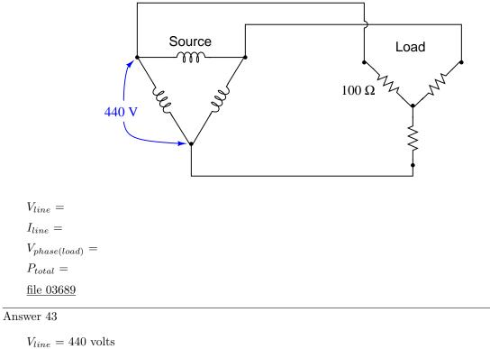
$V_{line} = 440$  volts  $I_{line} = 2.54$  amps  $V_{phase(load)} = 254$  volts  $P_{total} = 1.936$  kW
