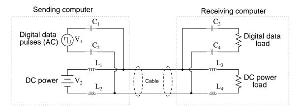
The system works fine for a while, but then one day the receiving computer stops receiving data. It still has DC power getting to it, but just no digital data. Identify the following:
