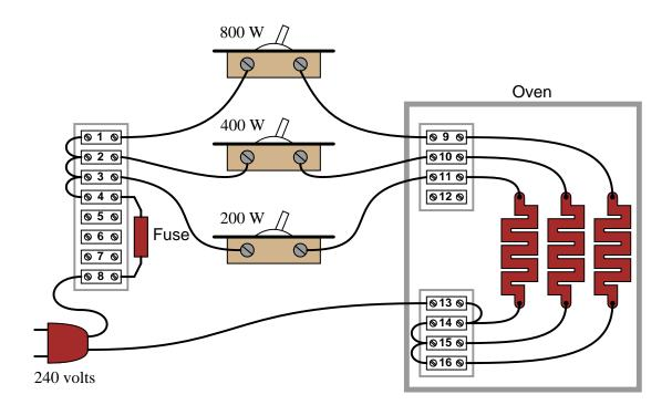
With three differently-sized heating elements (200 watt, 400 watt, and 800 watt), the oven operator can set the power in seven discrete steps by turning on specific combinations of switches: 200 watts, 400 watts, 600 watts, 800 watts, 1000 watts, 1200 watts, and 1400 watts.
