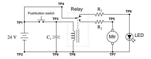
However, a problem has developed with this circuit. Neither the motor nor the green LED ever energizes, no matter what is done with the pushbutton switch. Strangely enough, the relay *does* make a "click" sound when the pushbutton is pressed, and then another "click" sound about 5 seconds after the switch is released. Based on this information, determine the following:
