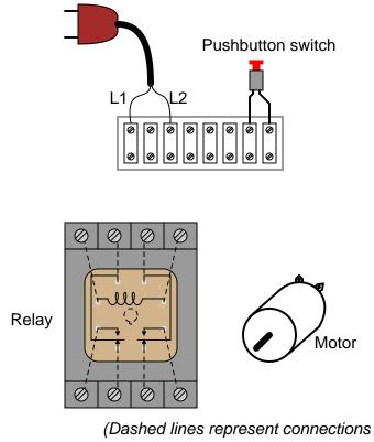
between relay terminals and socket screw lugs, hidden from sight)
