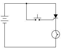
Insert a second switch into the schematic diagram that allows someone to de-energize the lamp once it has been "latched" on by actuating the first switch.
