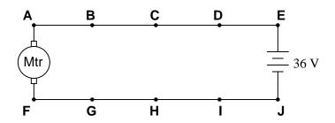
Connecting your voltmeter between points  $\mathbf{B}$  and  $\mathbf{G}$  in the circuit, you measure 36 volts as well. What does this indicate about the location of the fault? Assume there is only *one* thing wrong with this circuit (no multiple faults!).
