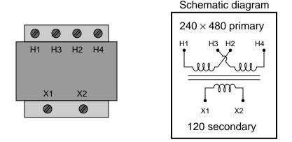
According to the person who did the field troubleshooting, the transformer is simply "bad." As is typical, you were given no other information to help diagnose the precise fault. Describe how you would test this transformer in your shop for the following faults, noting the transformer terminals you would connect your multimeter to and the type of meter measurement you would expect to see for each specified fault.
