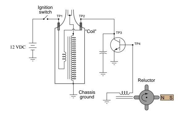
You are then asked to look at the circuit to see if you can figure out what is wrong. Using your multimeter, you measure voltage between TP1 and ground (12 volts DC) and also between TP2 and ground (0 volts DC). These voltage readings do not change at all as the reluctor spins.
