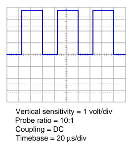
Calculate the duty cycle of this waveform, and also the average power dissipated by the load assuming a load resistance of 10.3  $\Omega.$
