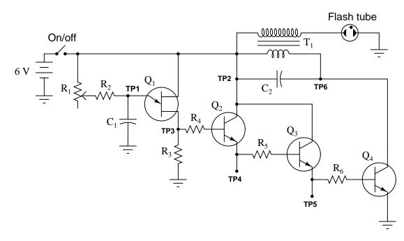
Turning the flash rate control (rheostat  $R_1$ ) to the slowest position, you take two voltage measurements with a voltmeter: at test point 3 (between TP3 and ground) you measure a voltage rhythmically pulsating between about 1.5 and 4 volts DC. At test point 6 (between TP6 and ground) you measure 6 volts DC all the time.
