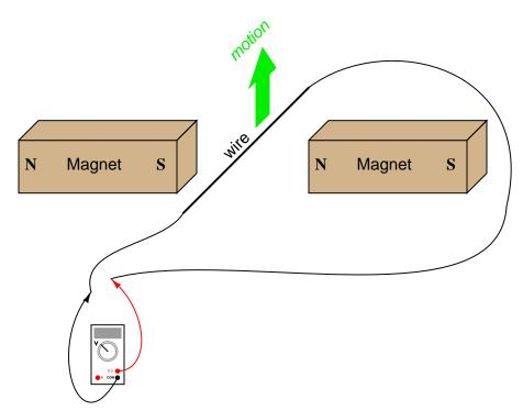
Describe the factors influencing the magnitude of the voltage induced by motion, and determine whether this is an example of an electric *motor* or an electric *generator*.  $\frac{file\ 00806}{file\ 00806}$
