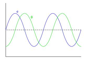
Based on this fact, draw the position of the magnetic rotor in this alternator when the voltage is at one of its peaks:
