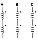
If one end of each winding pair were connected together at a common ground point, and each winding pair output 70 volts RMS, how much voltage would be measured between any two open wires?
