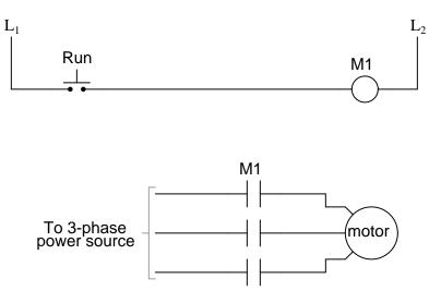
Also, explain the operation of this motor control circuit. What happens when someone actuates the "Run" switch? What happens when they let go of the "Run" switch? file 00834
