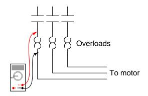
Across each overload heater element he measures about 20 mV AC with the starter engaged. From this he determines that the motor is *not* single-phasing, but is drawing approximately equal current on all three phases.
