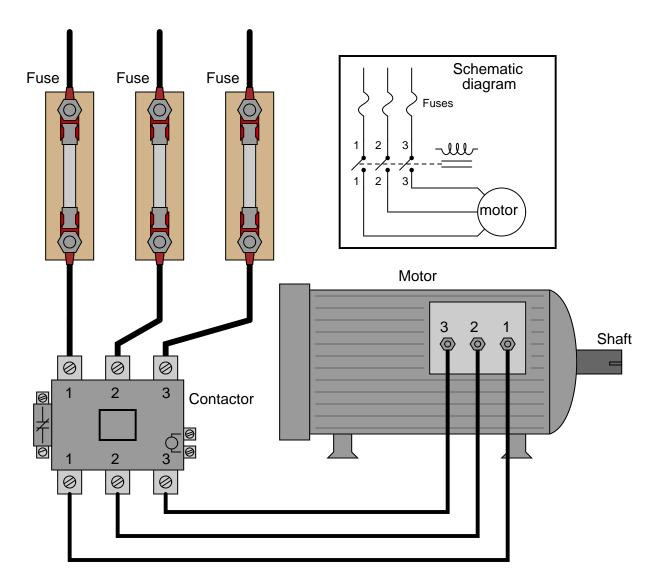
After years of faithful service, one day this motor refuses to start. It makes a "humming" sound when the contactor is energized (relay contacts close), but it does not turn. A mechanic checks it out and determines that the shaft is not seized, but is free to turn. The problem must be electrical in nature!
