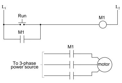
Also, explain the operation of this motor control circuit. What happens when someone actuates the "Run" switch? What happens when they let go of the "Run" switch? file 00835
