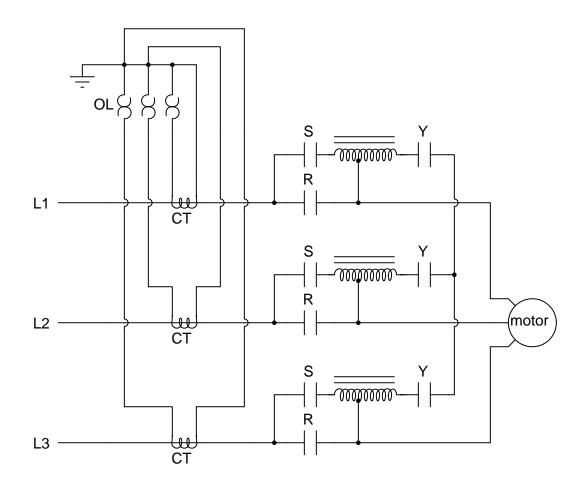
"L1," "L2," and "L3" represent the three phase power supply conductors. Three sets of contacts (R, S, and Y) serve to connect power to the motor at different times. The starting sequence for the motor is as follows:
