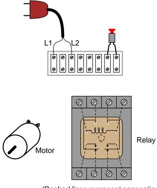
(Dashed lines represent connections between relay terminals and socket screw lugs, hidden from sight)
