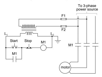
Explain the operation of this circuit, from the time the "Start" switch is actuated to the time the "Stop" switch is actuated. The normally-open M1 contact shown in the low-voltage control circuit is commonly called a *seal-in contact*. Explain what this contact does, and why it might be called a "seal-in" contact. file 01347
