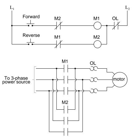
Explain how the reversal of motor direction is accomplished with two different motor starters, M1 and M2. Also, explain why there is only one set of overload heaters instead of two (one for forward and one for reverse). Finally, explain the purpose of the normally-closed contacts in series with each starter coil. file 03142
