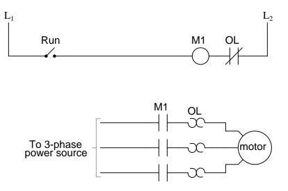
Although the "heater" elements are connected in series with the motor lines as fuses would be, they are *not* fuses! In other words, it is not the purpose of an overload heater to burn open under an overcurrent fault condition, although it is possible for them to do so.
