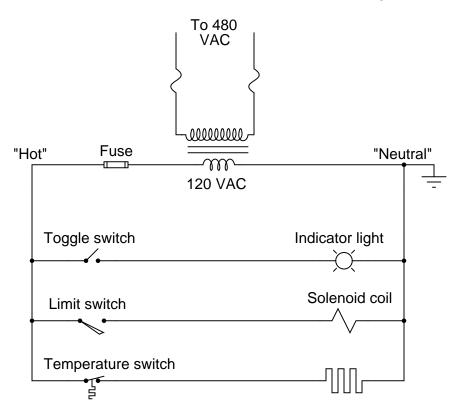
As you can see, the symbolism in ladder diagrams is not always the same as in electrical schematic diagrams. While some symbols are identical (the toggle switch, for instance), other symbols are not (the solenoid coil, for instance).
