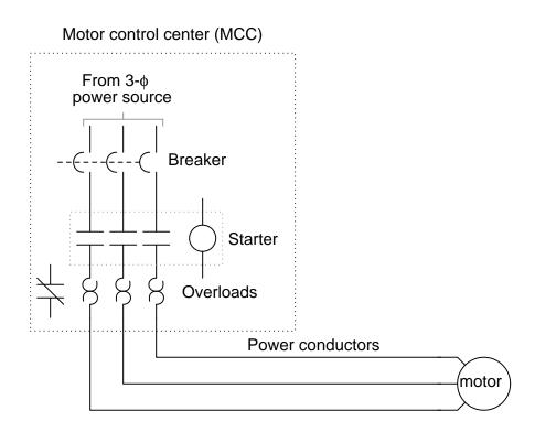
Since it is impossible for a technician to be in two places at once, it is often necessary to perform diagnostic checks on a malfunctioning electric motor from the MCC where the technician has access to all the control circuitry.
