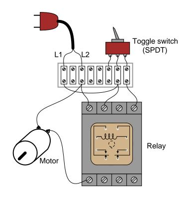
Challenge question: which switch position (handle to the left or handle to the right) turns the motor on?
