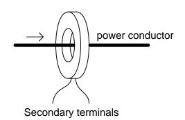
The purpose of a current transformer is to create a secondary current that is a precise fraction of the primary current, for easier measurement of current in the power conductor.
