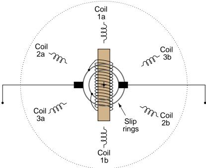
Explain how this motor can be operated as either a synchronous motor or a "plain" induction motor. file 00741
