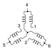
There are six terminals on the motor itself where the connections are made:
