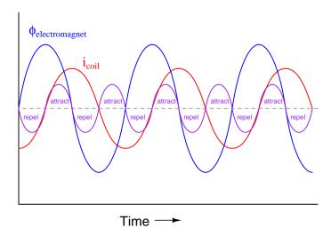
Note the equal-amplitude attraction and repulsion peaks shown on the graph.
