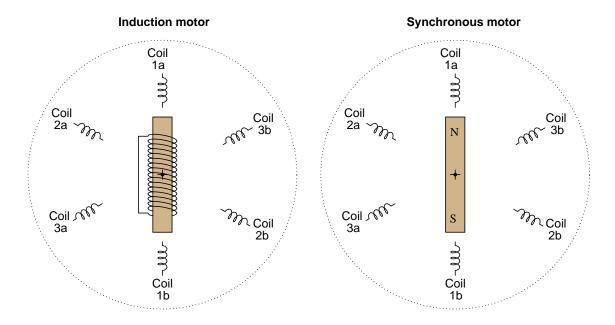
Synchronous AC motors use a permanent magnet rotor, while *induction* motors use an electromagnet rotor. Explain what practical difference this makes in each motor's operation, and also explain the meaning of the motors' names. Why is one called "synchronous" and the other called "induction"?
