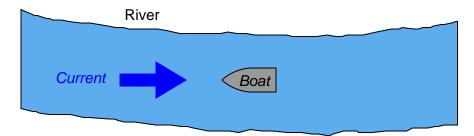
Suppose the driver of this boat does not own an anchor, and furthermore that the only form of propulsion is an electric "trolling" motor with an on/off switch (no variable speed control). With the right combination of switch actuations (on, off, on, off), it should be possible for the boat to maintain its position relative to the riverbanks, against the flow of water.
