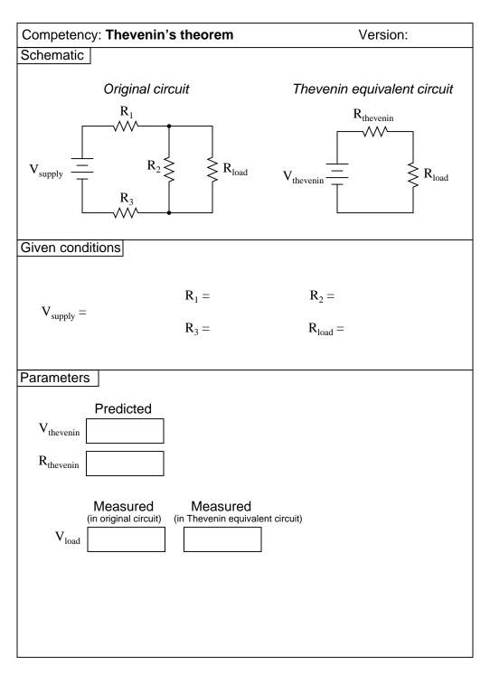
Use circuit simulation software to verify your predicted and measured parameter values.
