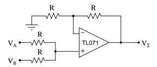
These two circuits perform the same mathematical function, yet the manners in which they perform this function are quite different. Compare and contrast the digital adder and the analog summer circuits shown here, citing any advantages or disadvantages of each.
