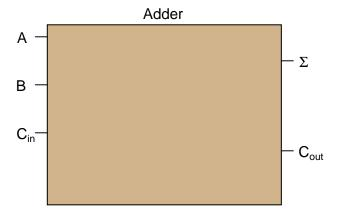
Begin the design process by drawing a truth table for the circuit, writing a boolean SOP expression for each output, then determining the necessary gate circuitry to fulfill each output function.
