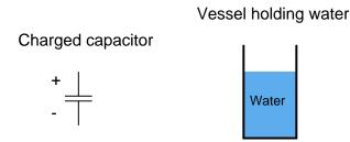
Complete this analogy, relating the electrical quantities of charge (Q), voltage (E or V), and capacitance (C) to the quantities of water height, water volume, and vessel dimensions. file 00188
