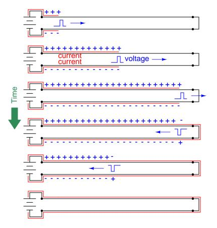
After the reflected pulse reaches the source, there will be minimum voltage at the source terminals and maximum current in the cable.
