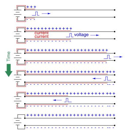
After the reflected pulse reaches the source, there will be maximum voltage at the source terminals and zero current in the cable.
