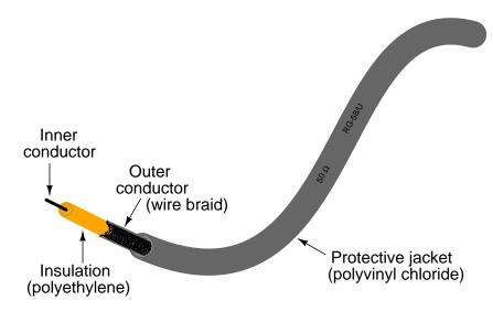
Note the "50 ohm" rating printed on the jacket of the cable. What will an ohmmeter register when connected between the inner conductor and shield of the cable? What will an ohmmeter register when connected between opposite ends of either the inner conductor or the shield, from one end of the cable to the other?
