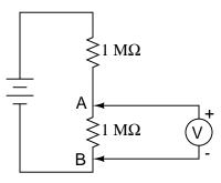
However, if you perform this same experiment using a real voltmeter, the measurement obtained with the meter will be substantially different from what *should* be there, based on a prediction of  $\frac{1}{2}E_{battery}$ . Explain why the voltmeter registers as it does. What is it about this circuit that causes the measurement to be so far off from the prediction, when we know full well that other voltage divider circuits we've constructed do not exhibit any significant error?
