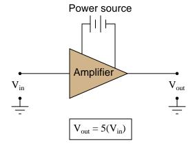
Translate this voltage gain ratio into a decibel figure. Explain why the conversion from voltage gain ratio to decibels is not the same as conversion of a power gain ratio to decibels.
