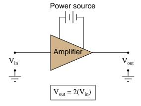
If we were to try to rate this amplifier's gain in terms of the relative power dissipated by a given load resistance ( $P_{load}$  when powered by  $V_{out}$ , versus  $P_{load}$  when powered by  $V_{in}$ ), what decibel figure would we calculate?
