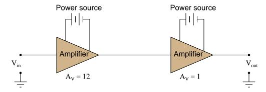
Also, convert the voltage gains of each amplifier into units of decibels, then convert the overall voltage gain ratio into units of decibels as well.
