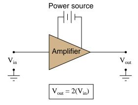
If we were to try to rate this amplifier's gain in terms of the relative *power* dissipated by a given load resistance ( $P_{load}$  when powered by  $V_{out}$ , versus  $P_{load}$  when powered by  $V_{in}$ ), what ratio would we calculate? In other words, what is the ratio of power for a given load resistance, when powered by a given voltage, versus when powered by a voltage that is twice as much?
