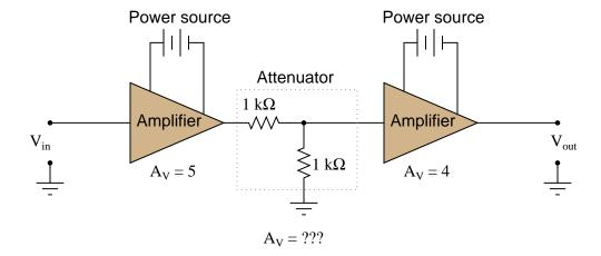
Also, convert the voltage gains of each stage into units of decibels, then convert the overall voltage gain ratio into units of decibels as well.
