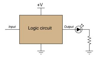
Complete this schematic diagram by including a switch in the drawing, such that in each of its two positions, a definite "low" or "high" logic state will be sensed by the circuit's input terminal.  $\underline{\text{file }01251}$
