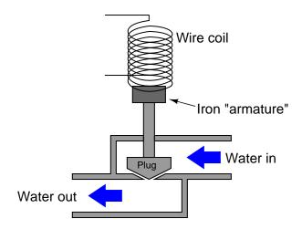
Essentially, this is an electrically-controlled on/off water valve. In the development of this valve, though, the design engineers discover that the magnetic force produced by the electromagnet coil is not strong enough to achieve reliable valve actuation every time. What can be changed in this solenoid valve design to produce a greater actuating force?
