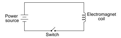
I will leave it to you to draw the illustration of this circuit on the crane. Your answer should show a wire *coil* embedded in the electromagnet assembly, a switch symbol near the operator, a battery symbol for the power supply, and wires carrying current to and from the electromagnet coil.
