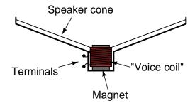
The "voice coil" is attached to the flexible speaker cone, and is free to move along the long axis of the magnet. The magnet is stationary, being solidly anchored to the metal frame of the speaker, and is centered in the middle of the voice coil.
