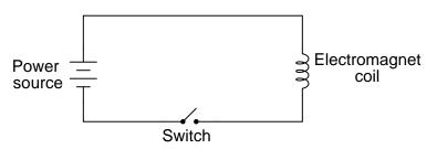
I will leave it to you to draw the illustration of this circuit on the crane. Your answer should show a wire *coil* embedded in the electromagnet assembly, a switch symbol near the operator, a battery symbol for the power supply, and wires carrying current to and from the electromagnet coil.
