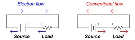
Whichever notation you choose to follow in your analysis of circuits, the understanding should be the same: the reason voltage polarities across the resistor and battery differ despite the same direction of current through both is the flow of power. The battery acts as a *source*, while the resistor acts as a *load*.
