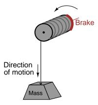
In each of the above scenarios, draw arrows depicting directions of two forces: the force that the mass exerts on the drum, and the force that the drum exerts on the mass. Compare these force directions with the direction of motion in each scenario, and explain how these directions relate to the mass and drum alternately acting as energy *source* and energy *load*.
