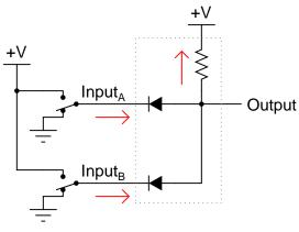
Current arrows pointing in the direction of electron flow!
