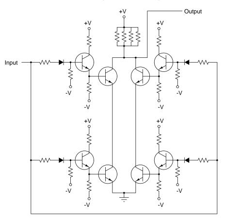
Explain why the circuit is referred to as *quad*-redundant. How many individual component failures, minimum, must occur before the gate's functionality is compromised? Prove your answer through an analysis of the circuit's operation.
