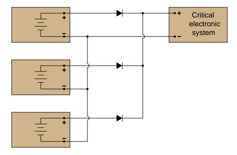
However, as an experienced electronics technician, you should know that diodes are not immune to failure. Modify this schematic diagram to include three extra (redundant) diodes that will allow normal operation if any one of the three original diodes were to fail, assuming the most common failure mode of rectifier-type diodes.
