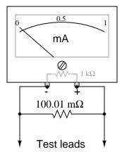
A power dissipation rating of at least 10 watts is necessary for this application.
