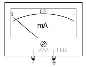
Show how a single resistor could be connected to this ammeter to extend its range to  $\theta$  to  $1\theta$  amps. Calculate the resistance of this "range" resistor, as well as its necessary power dissipation rating. file 00370
