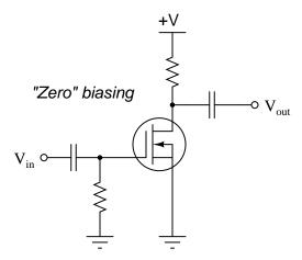
This may appear similar to self-biasing as seen with JFET amplifier circuits, but it is not. Zero biasing only works with IGFET amplifier circuits. Explain why this is so.
