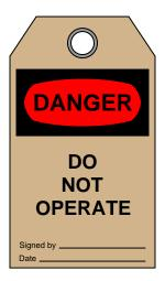
What is the purpose of attaching such a tag to an electrical disconnect device in addition to locking it in the open position? Why is a lock, by itself, not sufficient from a safety perspective?  $\frac{\text{file }00573}{\text{electrical}}$
