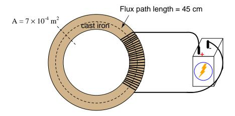
Calculate the amount of current necessary in the wire coil to establish this amount of flux, if the coil has 250 turns, and the torus has an average flux path length of 45 cm. Also, calculate the amount of magnetic flux  $(\Phi)$  inside the torus.
