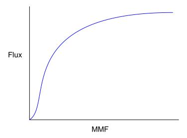
What does this graph indicate to you, as compared to the graph for a resistor's characteristics? What is the significance of this with regard to magnetic "circuit" analysis?
