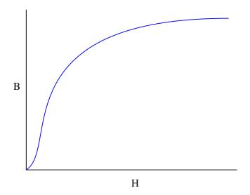
Rarely will you see a plot of flux  $(\Phi)$  shown as as a function of MMF  $(\mathcal{F})$ , even though such a plot would appear very similar to the "B/H curve" for that same material. Why is this? Why would a "B/H" curve be preferable to an engineer rather than a "Flux/MMF" curve?
