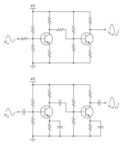
Which of these two designs would be more suitable for use in a DC voltmeter circuit (amplifying a measured DC voltage)? What applications would the *other* amplifier design be suited for? file 01119
