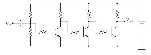
With no emitter swamping resistors anywhere in this circuit, the voltage gain of each stage is guaranteed to be large, but unstable as well. With three stages arranged like this, one feeding into the next, the final voltage gain will be very large, and very unstable.
