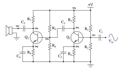
Explain a logical, step-by-step approach to identifying the source of the problem, by taking voltage signal measurements. Remember, the more efficient your troubleshooting technique is (the fewer measurements taken), the better!
