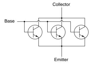
However, if transistors are directly paralleled as shown, reliability problems may develop. A better way of "ganging" multiple transistors together is to connect a low-value *swamping resistor* to each emitter terminal:
