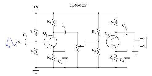
Which option would be better, and why? What ill effects could result from locating the potentiometer in the wrong place in this circuit?
