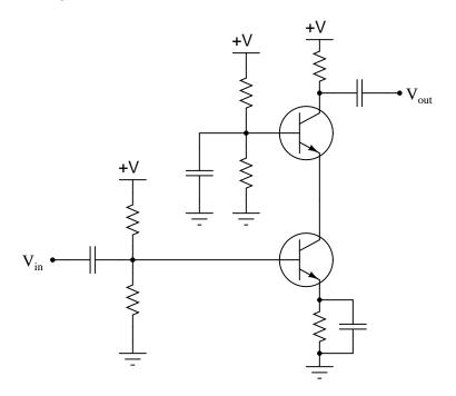
What advantage(s) does the cascode amplifier have over "normal" single- or multi-stage amplifier designs? What, specifically, makes it well suited for high-frequency applications, such as RF (Radio Frequency) signal amplifiers?
