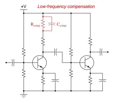
Explain how the presence of this "compensating" capacitor helps to overcome the loss of gain normally experienced as a result of the other capacitors in the circuit.
