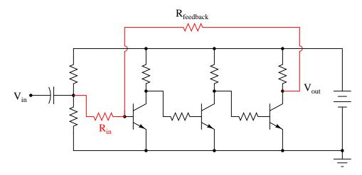
Interestingly, the voltage gain of such a circuit will be nearly equal to the quotient of the two highlighted resistors,  $R_{feedback}$  and  $R_{in}$ :
