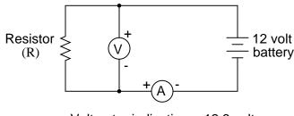
Voltmeter indication = 12.3 volts Ammeter indication = 4.556 milliamps
