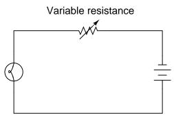
This method of electrical power control is not without its disadvantages, though. Consider an example where the circuit current is 5 amps, the variable resistance is 2  $\Omega$ , and the lamp drops 20 volts of voltage across its terminals. Calculate the power dissipated by the lamp, the power dissipated by the variable resistance, and the total power provided by the voltage source. Then, explain why this method of power control is not ideal.
