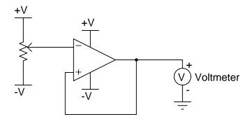
The output voltage will saturate at approximately +11 volts, or -11 volts, with the potentiometer having little or no effect.
