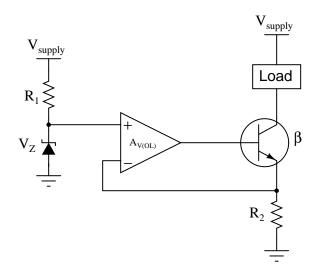
Write an equation solving for the regulated load current, given any relevant variables shown in the schematic diagram  $(R_1, V_Z, V_{supply}, A_{V(OL)}, \text{etc.})$ . file 02512
