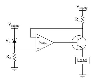
Explain how this op-amp really does provide *negative* feedback, which of course is necessary for stable current regulation, as positive feedback would be completely unstable.
