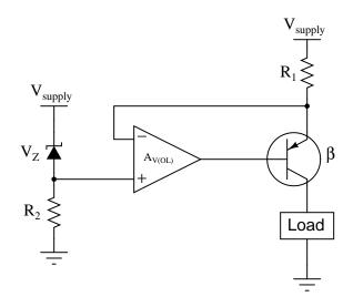
Write an equation solving for the regulated load current, given any relevant variables shown in the schematic diagram  $(R_1, V_Z, V_{supply}, A_{V(OL)}, \text{ etc.})$ . Also, describe what would have to be changed in this circuit in order to set the regulated current at a different value.
