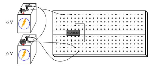
With the noninverting input connected to ground (the midpoint in the split +6/-6 volt power supply), the student expects to measure 0 volts DC at the output of the op-amp. This is what the DC voltmeter registers, but when set to AC, it registers substantial AC voltage!
