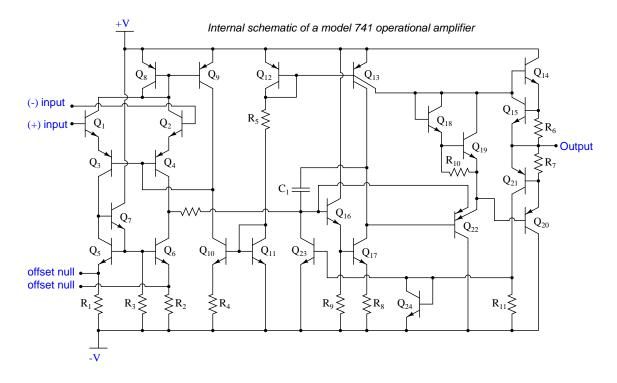
Explain how active loading creates the constant slew rate exhibited by operational amplifier circuits such as the 741. What factors account for the *linear* ramping of voltage over time? file 02603
