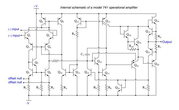
Find the compensation capacitor in this schematic diagram, and identify how it provides frequency-dependent negative feedback within the opamp to reduce gain at high frequencies.
