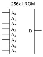
Suppose we wished to program this memory IC to act as a digital comparator, outputting a logical "high" state only when two four-bit binary numbers are equal:
