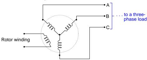
How much AC voltage will appear between any two of the lines  $(V_{AB}, V_{BC}, \text{ or } V_{AC})$  if each stator coil inside the alternator outputs 277 volts? Draw a phasor diagram showing how the phase (winding) and line voltages relate.
