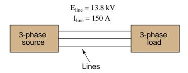
A 13.8 kV single-phase system could be designed to provide the same amount of power to a load, but it would require heavier-gauge (more expensive!) conductors. Determine the extra percentage of expense in wire cost (based on the weight of the wires) resulting from the use of single-phase instead of three-phase.
