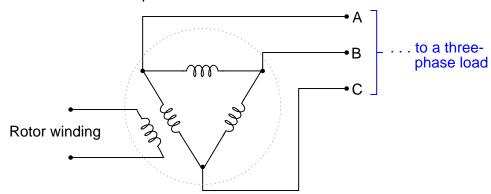
How much AC current will each of the lines  $(I_A, I_B, \text{ or } I_C)$  conduct to a load (not shown) if each stator coil inside the alternator outputs 17 amps of current?
