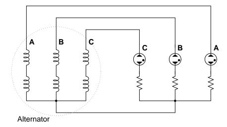
If the alternator spins fast enough (clockwise, as shown), the AC voltage induced in its windings will be enough to cause the neon lamps to "blink" (neon bulbs have very fast reaction times and thus cannot maintain a glow for very long without current, unlike incandescent lamps which operate on the principle of a glowing-hot metal filament). Most likely this blinking will be too fast to discern with the naked eye.
