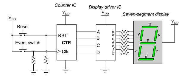
Please note that this is only a general schematic, and that the details will vary according to the particular chips you happen to choose. For example, the counter may be positive edge-triggered or negative edge-triggered; its reset may be active-high or active-low; if it is a binary counter (not BCD), you will have to add at least one logic gate to truncate its count from 0-F (hex) to 0-9 (BCD); the display driver may require common-anode or common-cathode displays; etc.
