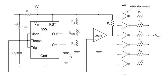
Here, six CMOS inverters (IC part number 4049) are ganged together in parallel to supply significantly more sourcing and sinking current capability than the LM339-with-pullup-resistor could on its own. Since CMOS logic gates are inherently on-or-off devices, they have no trouble handling the square wave output of the LM339.
