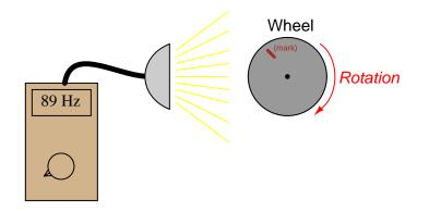
A second technician comes along and disagrees with the first. According to the second, more testing is required before it can be sure that the wheel's speed is actually 600 RPM. The first technician is perplexed: how can the speed be anything *but* 600 RPM, if 10 Hz is the strobe frequency where the mark is seen to "stand still?"
