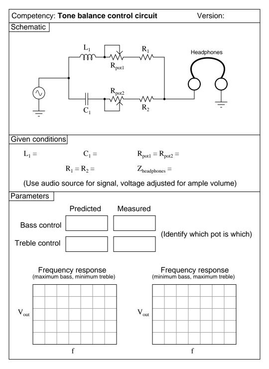
Note: when testing the frequency response of the tone control circuit, you may need to replace the headphones with a non-inductive resistor of equivalent impedance, and measure  $V_{out}$  across it. file 02022
