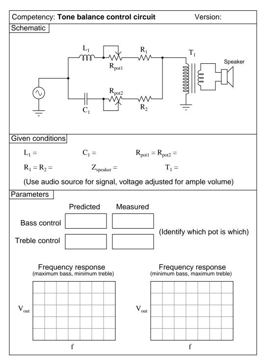
Note: when testing the frequency response of the tone control circuit, you may need to replace the transformer/speaker assembly with a non-inductive resistor of equivalent impedance, and measure  $V_{out}$  across it.
