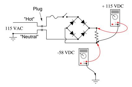
Challenge question: how could the 58 volts from (-) to ground be eliminated, so as to permit grounding of the (-) output terminal?
