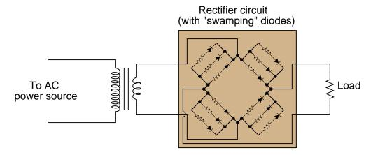
Explain why these resistors are necessary to ensure long diode life.
