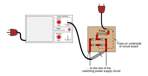
However, the technician is surprised to find that the fuse blows every time she turns the power on to the circuit. When the oscilloscope is disconnected from the circuit, the fuse does not blow, and everything works fine. What is wrong? Why does the oscilloscope cause a fault in the circuit?
