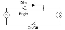
Explain how this circuit is able to make the light bulb glow brighter and dimmer.  $\underline{\text{file }00782}$
