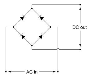
Draw the connections in this illustration to form a bridge rectifier circuit, receiving power from the transformer and delivering power to the light bulb:
