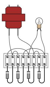
Follow-up question: draw the direction of currents through the bridge rectifier for each half-cycle of the AC power source, and determine the DC voltage polarity across the light bulb terminals.
