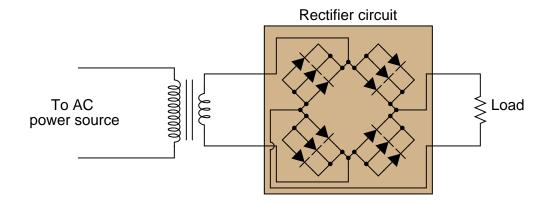
Follow-up question: while this circuit should work (in theory), in practice one or more of the diodes will fail prematurely due to overheating. The fix for this problem is to connect "swamping" resistors in series with the diodes like this:
