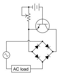
Explain how this circuit functions. How is the transistor (a DC-only device) able to control alternating current (AC) through the load?
