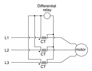
Also, explain what this relay will do to protect the circuit if it detects this kind of fault.  $\underline{file~04024}$
