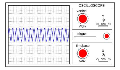
What display control(s) need to be adjusted on the oscilloscope in order to show fewer cycles of this signal on the screen, with a greater height (amplitude)?
