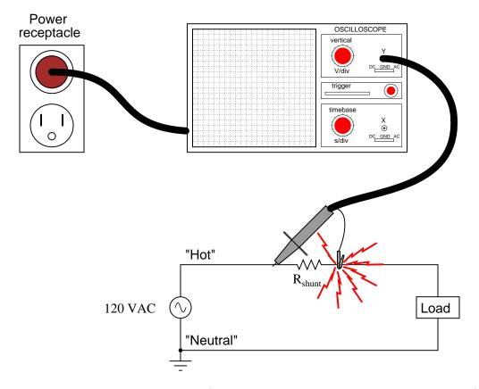
Here, the reference lead of the oscilloscope (the small alligator clip, not the sharp-tipped probe) creates a short-circuit in the power system. Explain why this happens.
