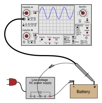
Setting the coupling control to "AC", however, results in the waveform automatically centering itself on the screen, about the zero line.
