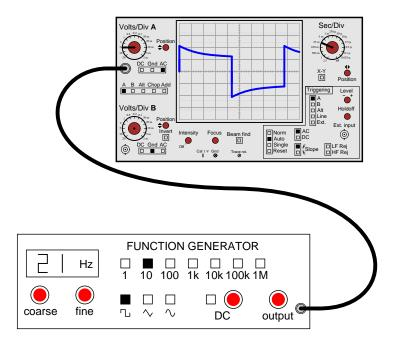
As you can see, the function generator is configured to output a square wave, but the oscilloscope does not register a square wave. Perplexed, the student takes the function generator to a different oscilloscope. At the second oscilloscope, the student sees a proper square wave on the screen:
