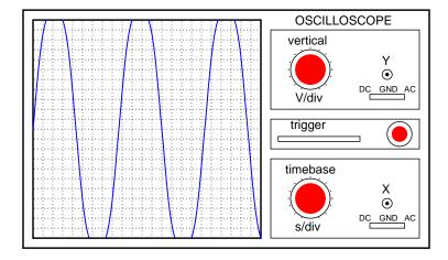
What display control(s) need to be adjusted on the oscilloscope in order to show a normal-looking wave on the screen?
