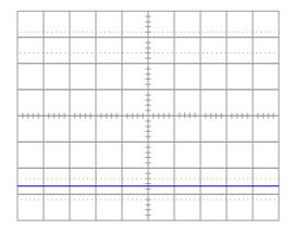
Assuming the oscilloscope display has been properly "zeroed" and the vertical sensitivity is set to 2 volts per division, determine the voltage of the battery.
