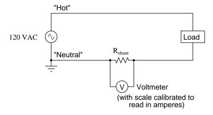
Since the schematic shows a shunt resistor being used to measure current in an AC circuit, it would be equally appropriate to use an oscilloscope instead of a voltmeter to measure the voltage drop produced by the shunt. However, we must be careful in connecting the oscilloscope to the shunt because of the inherent ground reference of the oscilloscope's metal case and probe assembly.
