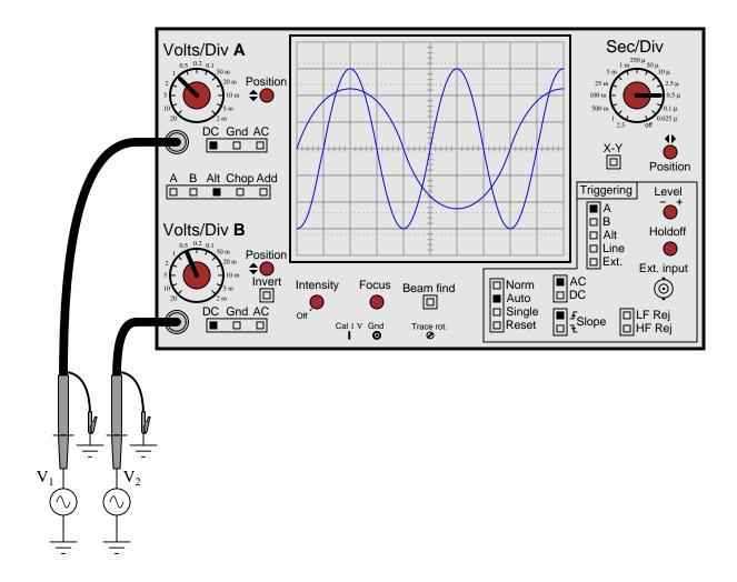
While this feature is extremely useful, one must be careful in connecting two sources of AC voltage to an oscilloscope. Since the "reference" or "ground" clips of *each* probe are electrically common with the oscilloscope's metal chassis, they are electrically common with each other as well.
