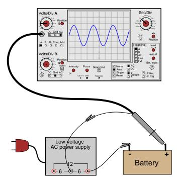
Based on these observations, explain what the "DC" and "AC" settings on the coupling control actually mean.
